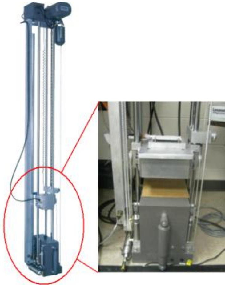
Figure 5.21: Experimental set-up for controlled JEDEC drop test using LANSMONT™ drop test tower.
