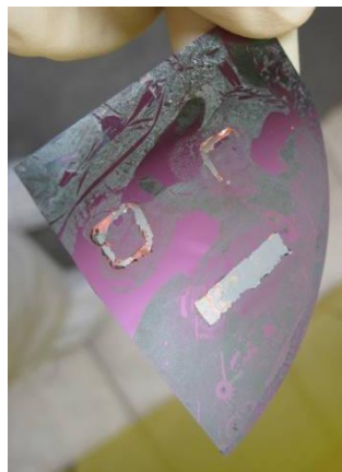
Figure 46: Wafer Quarter Post-PR Removal (back)
