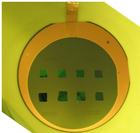
Figure 37: Sample Dicing Tape Incision
