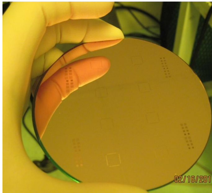
Figure 62: Wafer Post-Copper Deposition
