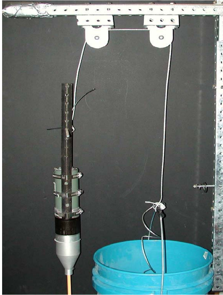
Figure 9. Pull test pulley system.
