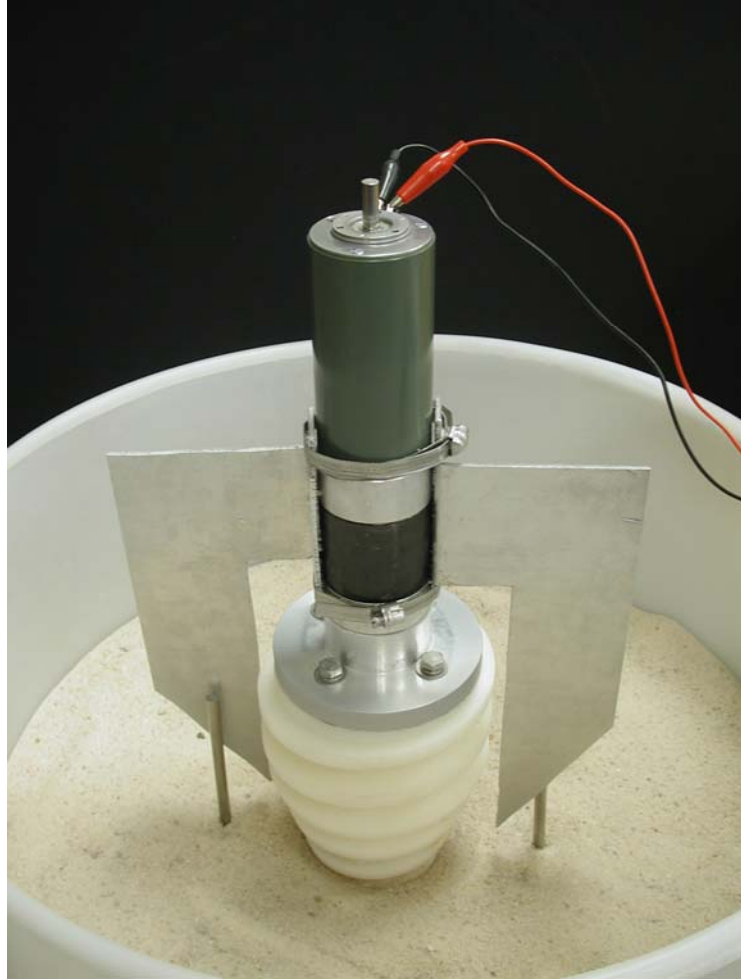
Figure 3. View of machined attachment connecting the conical auger to the motor.
