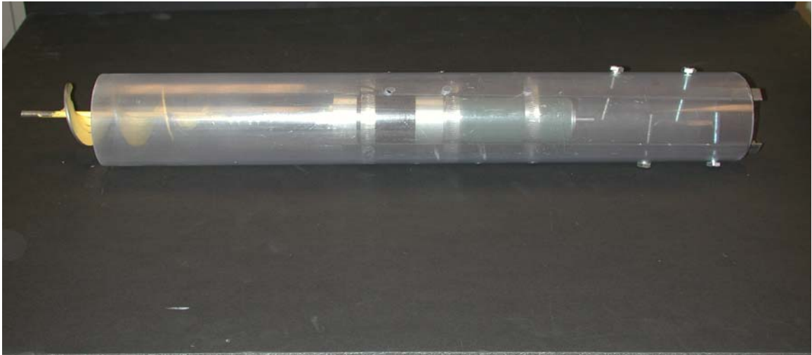
Figure 12. Earthworm design; Motor and 76 mm auger within a tube.
