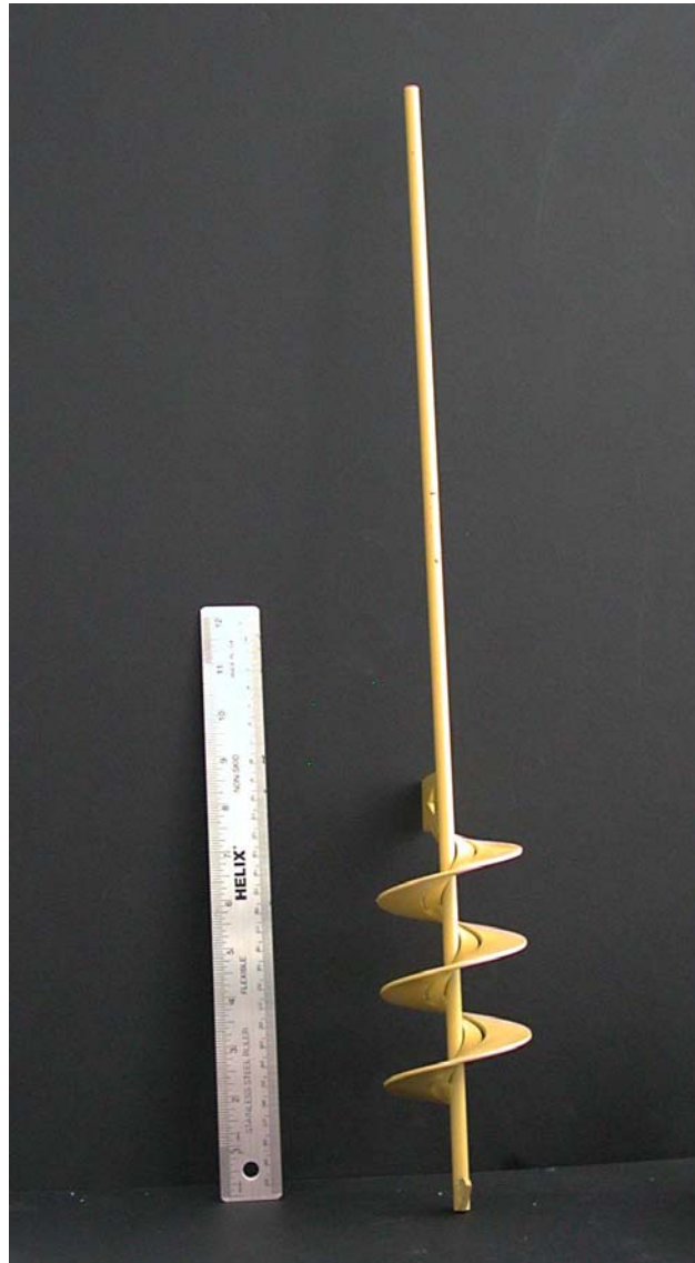
Figure C-1. Extended auger used for pull test
