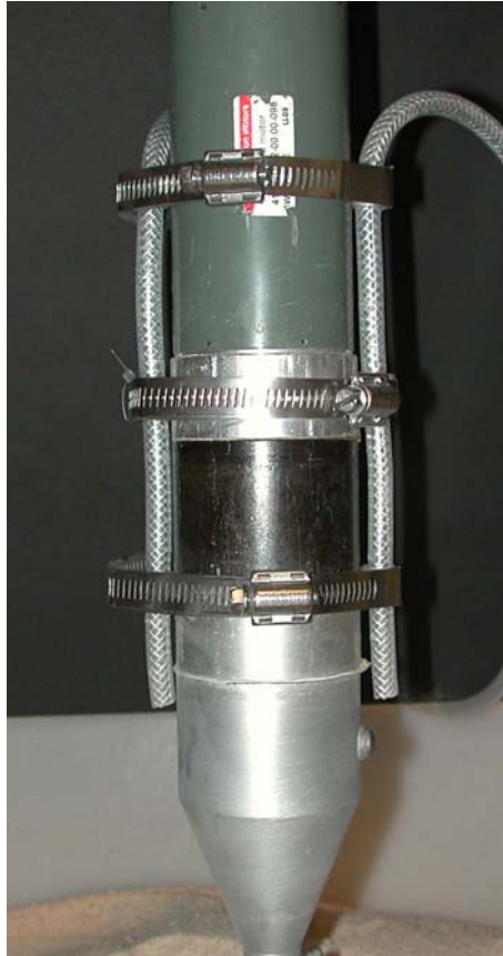
Figure 19. Visual of motor with air hoses to help reduce the surface friction.
