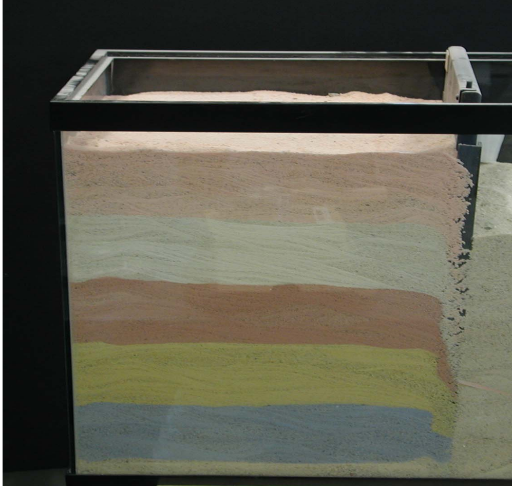
Figure 10. Multi colored sand used to examine the auger-sand interactions.
