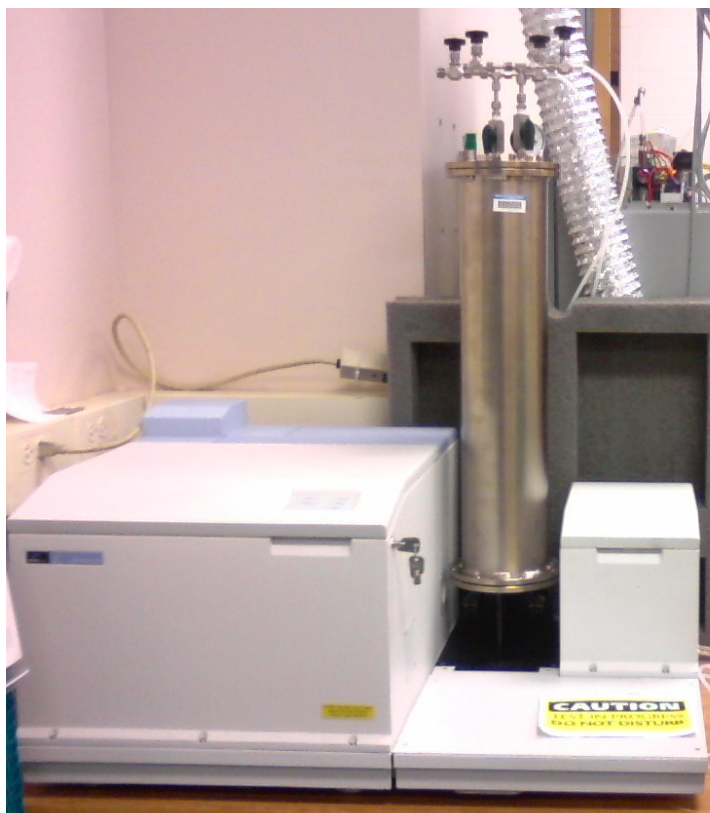
Figure 2-6: Laboratory Test Environment, FTIR Gas Analysis Module with Spectrum GX FTIR (Perkin Elmer, Shelton, CT, USA) with M-5-22-V Variable Pathlength Long Path Gas Cell (Infrared Analysis, Inc., Anaheim, CA, USA)
