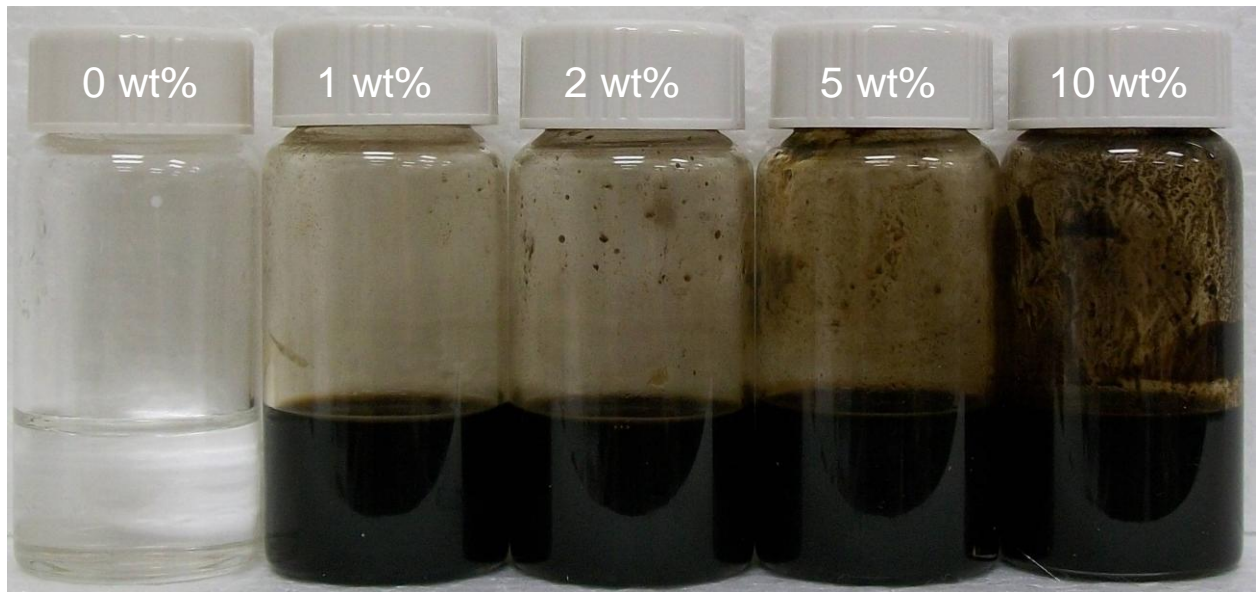
Figure 3.4 Photograph of eicosane-based NePCM samples (in liquid phase) with various mass fractions (0, 1, 2, 5 and 10 wt%) of CuO nanoparticles
