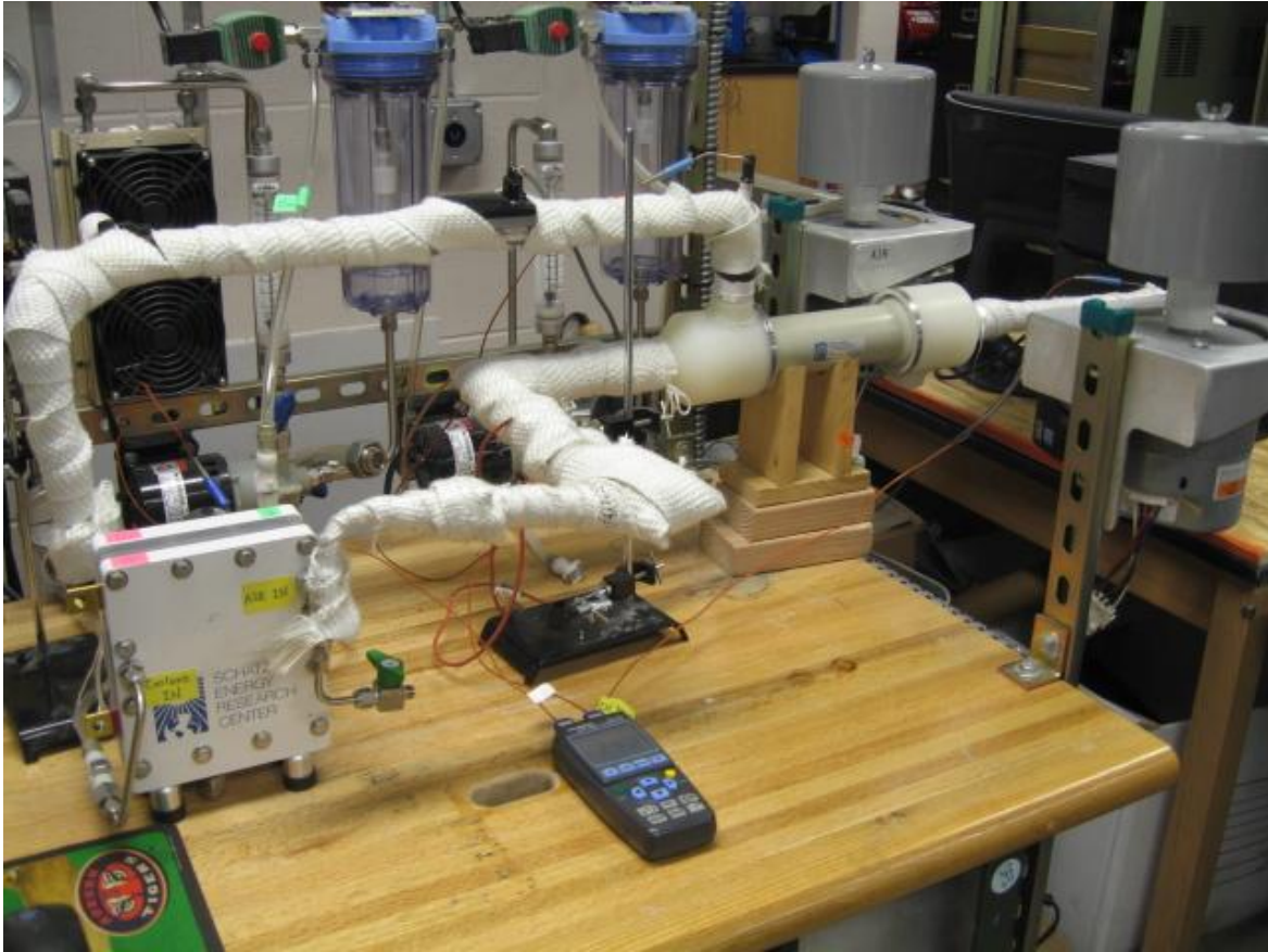
Figure 3-26. Fuel cell test station.
