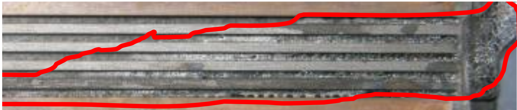
Figure 4.6 Liquid water distribution along GFCs for different inlet RH of air.
