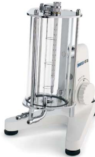
Figure 1.6. Schematic of falling sphere viscometer (from Brookfield Engineering Laboratories, Inc. [31])
