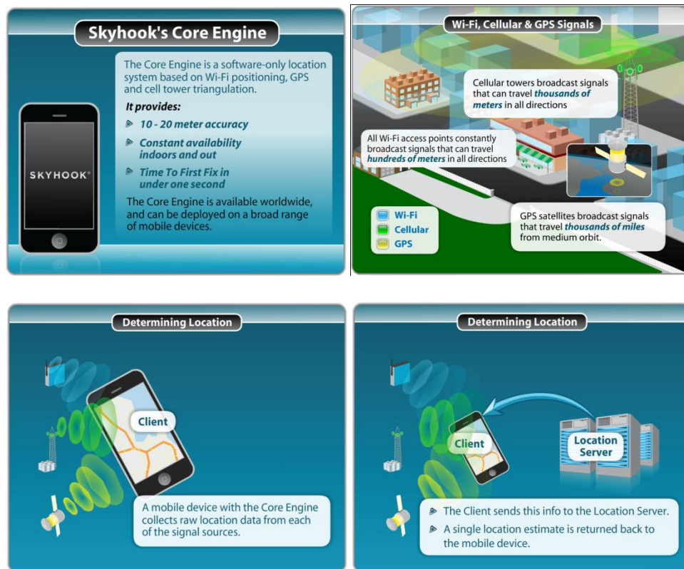
Figure 20 Description of Wi-Fi localization from Skyhook Wireless (Skyhook Wireless, 2011)
