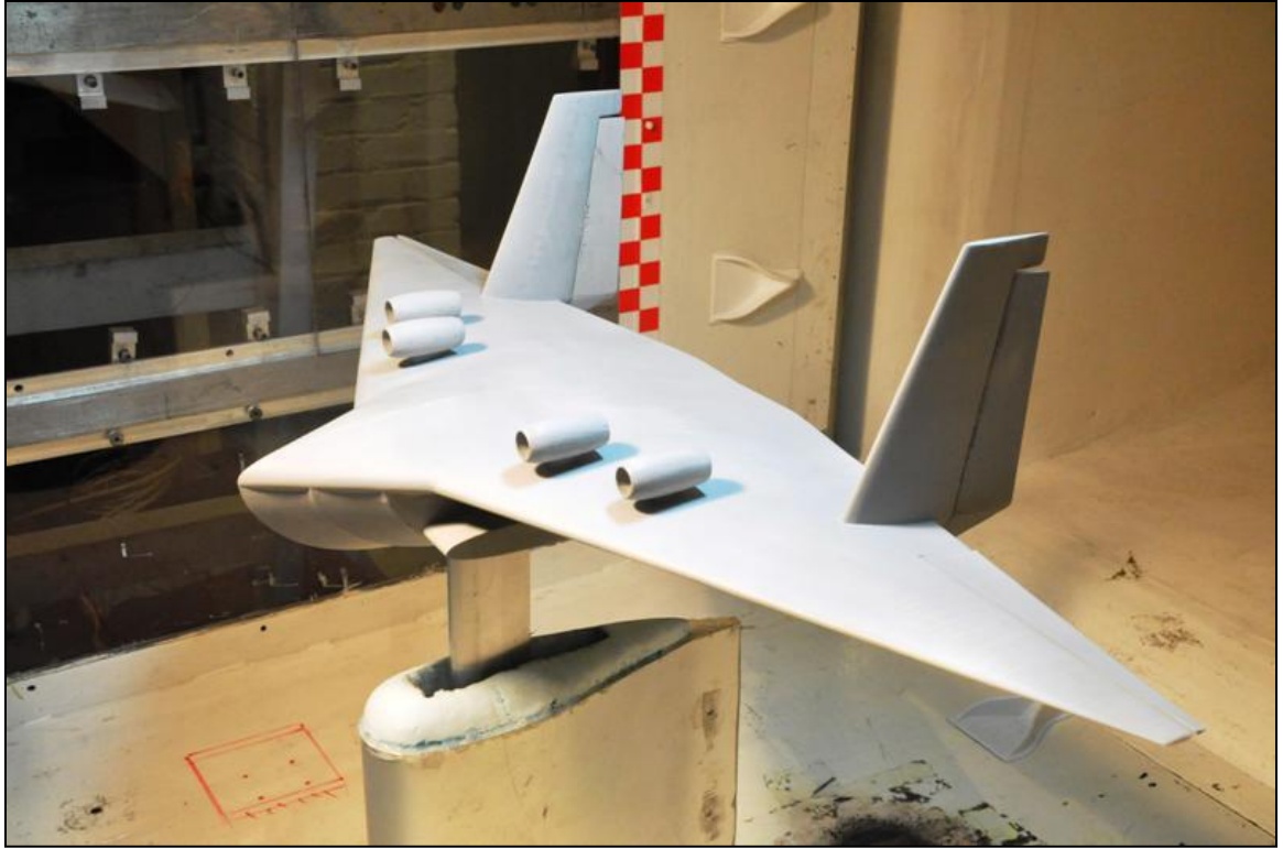
Figure 36: Wind Tunnel Model, Mounting Blade and Shroud
