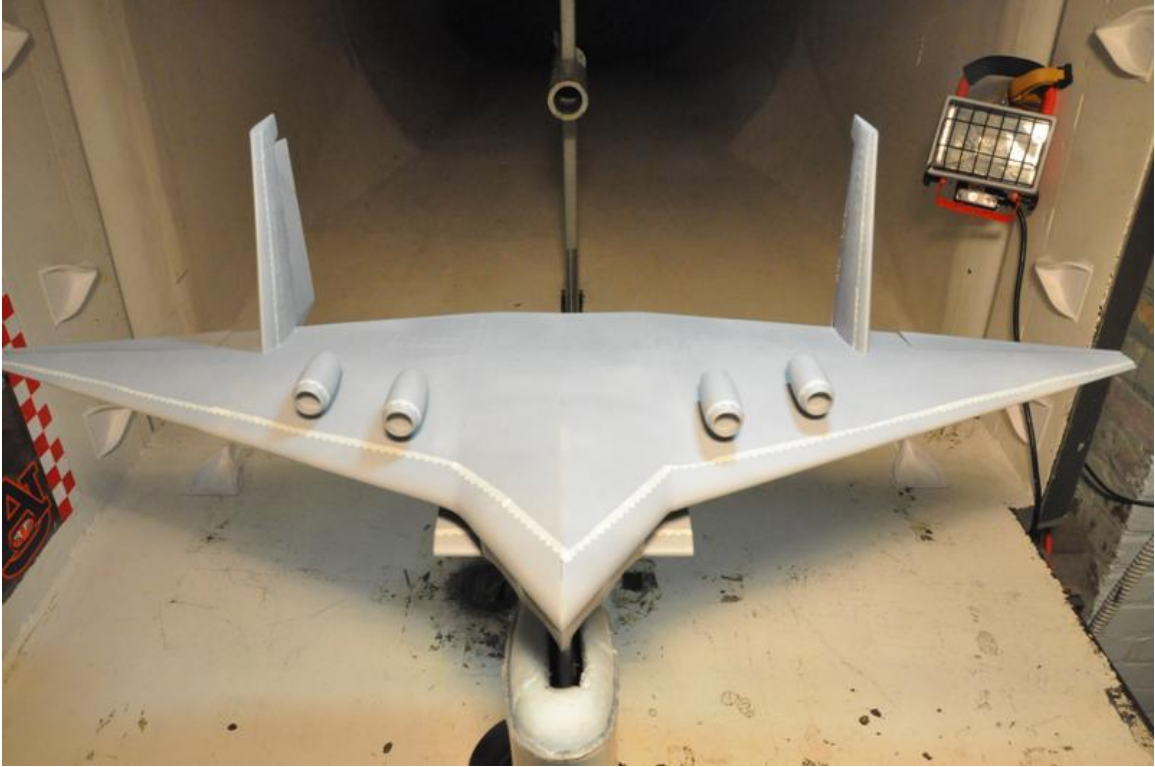
Figure 44: Wind Tunnel Model with Transition Strip
