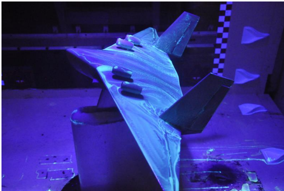
Figure 49: Flow Visualization - 20 Degree AoA - No Strip
