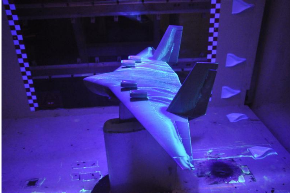
Figure 47: Flow Visualization - 5 Degree AoA - No Strip
