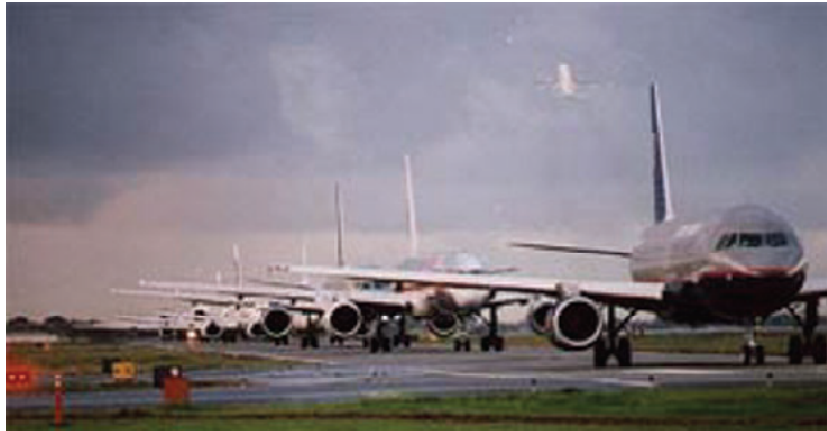
Figure-1.4 Wake-vortex separation requirements under instrument flight rules conditions aggravate airport capacity problem [3].
