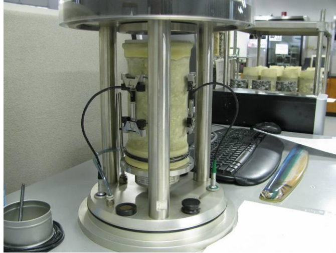
Figure 5.6 Dynamic Modulus Specimen in AMPT
