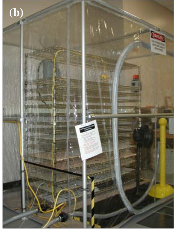
Fig. 33. Experimental setup of (a) Steris 1000ED bio-decontamination unit attached to a small stainless steel enclosure for precise control of vapor concentration and (b) walk-in tent enclosure for large number of specimens processing.
