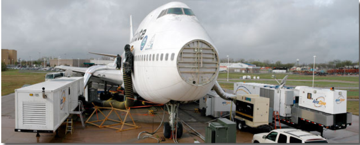
Fig. 1. Demonstration of decontamination of entire wide body airliner cabin using vapor phase hydrogen peroxide at Oklahoma City, OK., USA, March 2007 [21].
