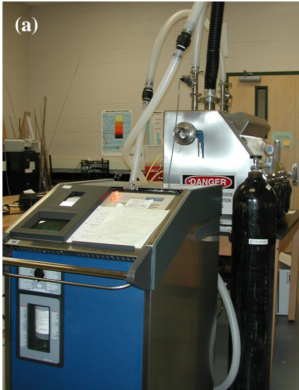
Fig. 33. Experimental setup of (a) Steris 1000ED bio-decontamination unit attached to a small stainless steel enclosure for precise control of vapor concentration and (b) walk-in tent enclosure for large number of specimens processing.
