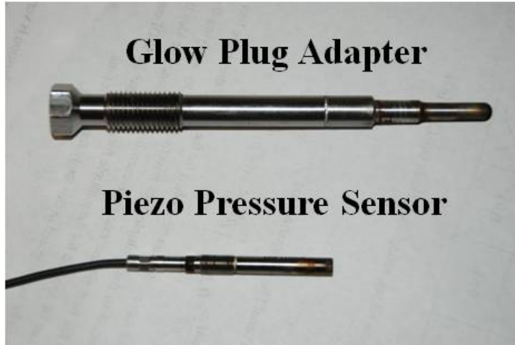
Figure 4 - 5: Kistler Pressure Sensor and Glow Plug Adapter
