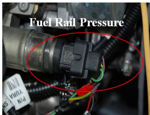
Figure 4 - 4: Fuel Rail Pressure Sensor Location
