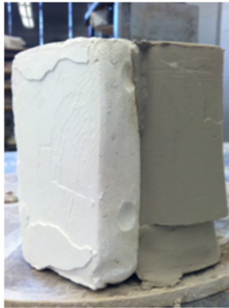
Figure 4.14: Take the mold apart
