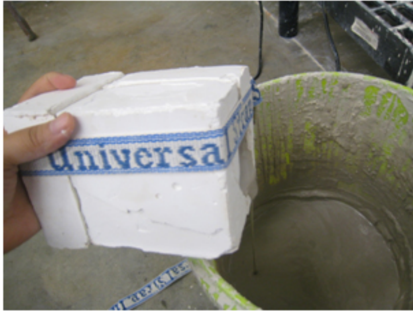
Figure 4.13: Pour excess slip out from the mold
