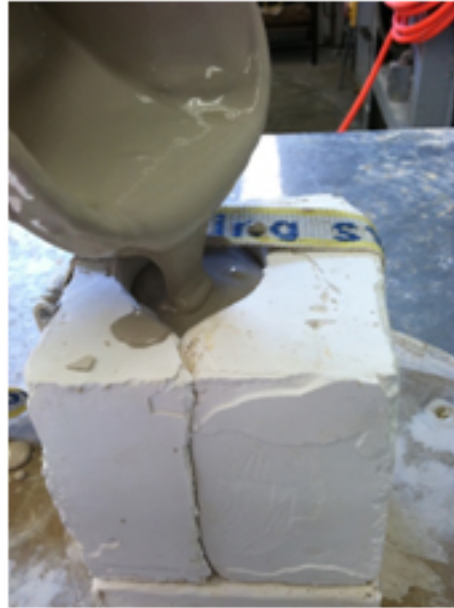
Figure 4.12: Pour the slip until the mold is full
