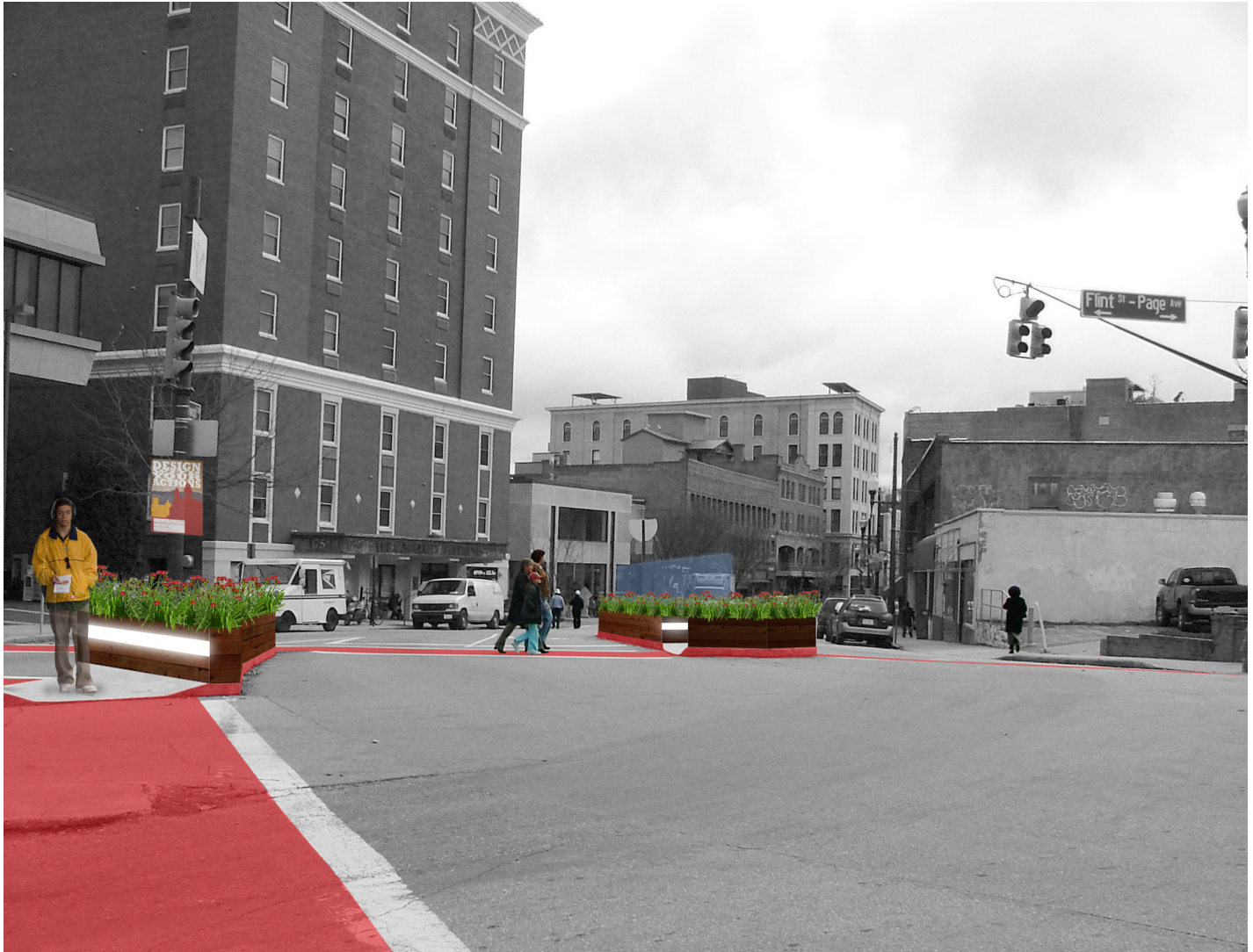
2.34 Haywood Street Calibration Highlighting the designated pedestrian paths and placing lighted planter boxes attempted to create better conditions for pedestrians crossing the intersection.
