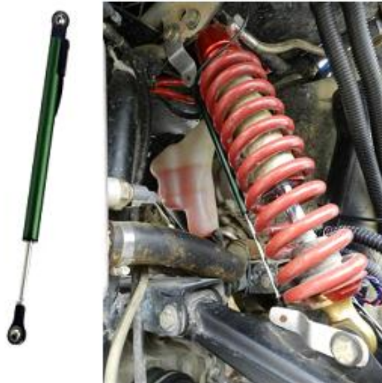
Figure C.5 – (left) Celesco MLP-125 linear potentiometer (right) mounting of potentiometer parallel to suspension coilovers.
