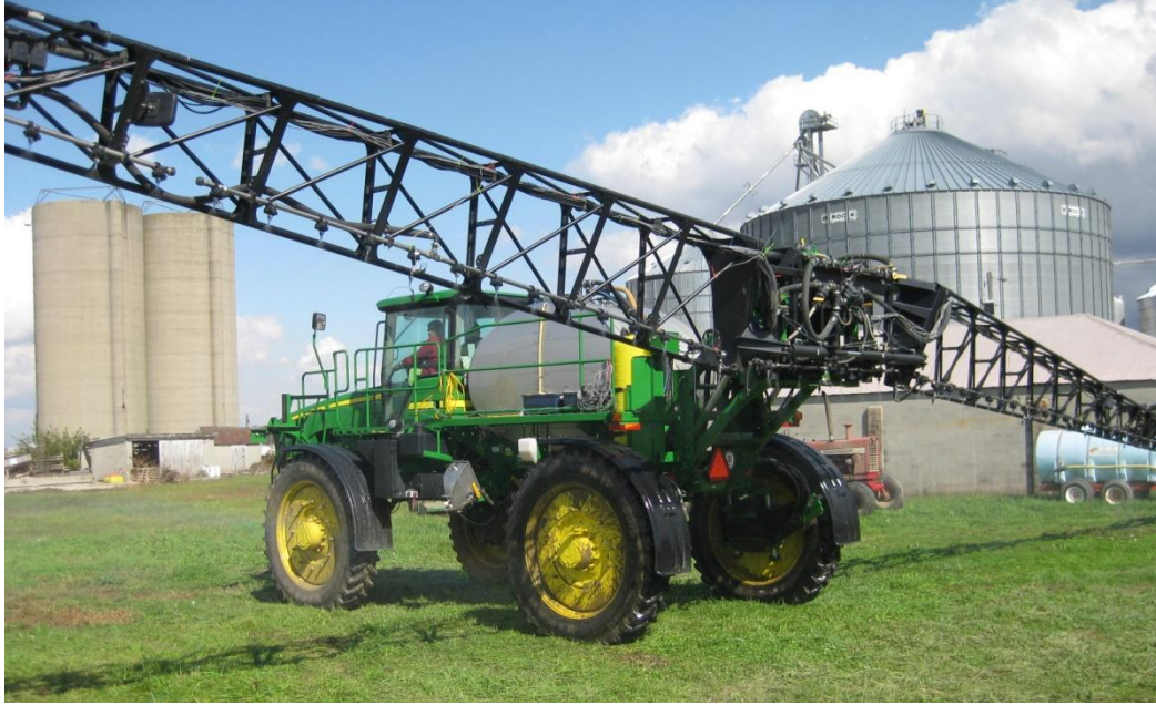
Figure B.1. Nozzle pressure measurement with left boom-section tilted upwards and right tilted downwards.
