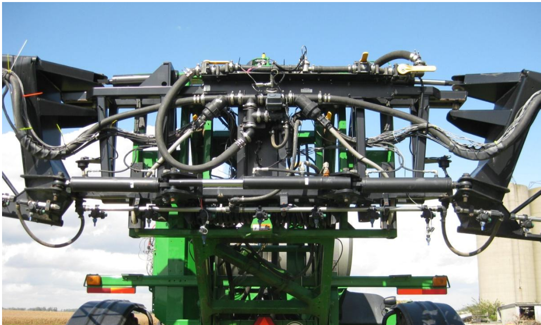
Figure B.2. Nozzle plumbing in the central boom-section.
