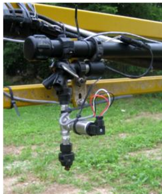
Figure 3.3. Pressure transducer mounted at a nozzle.
