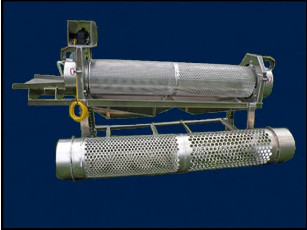
Figure 2.7A. Image of the QuickTube Sorter™ rotary grader and the interchangeable grading tubes. Image credit: Chesapeake Bay Oyster Company.
