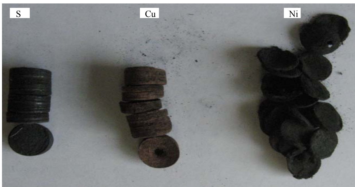
Figure V-7. Spent SS, Cu, and Ni MFEC structures. SS and Cu fibers were stable, Ni fibers showed significant deterioration
