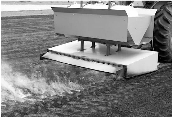
Figure 1. PL8750 flame sanitizer demonstrating short-term thermal heat exposure period. Red Dragon, Model PL8750 Poultry House Flame Sanitizer, Flame Engineering, Inc. P.O. Box 577 LaCrosse, Kansas 67548
