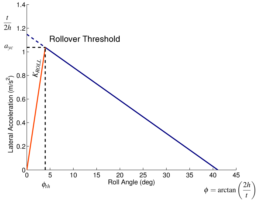
Figure 5.16: Method of determining rollover index thresholds.
