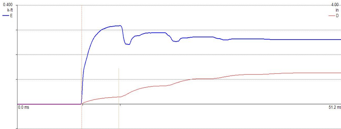
Figure 2.6 EFV & E-D Trace-Long Rod (49.3 ft)-low penetration resistance
