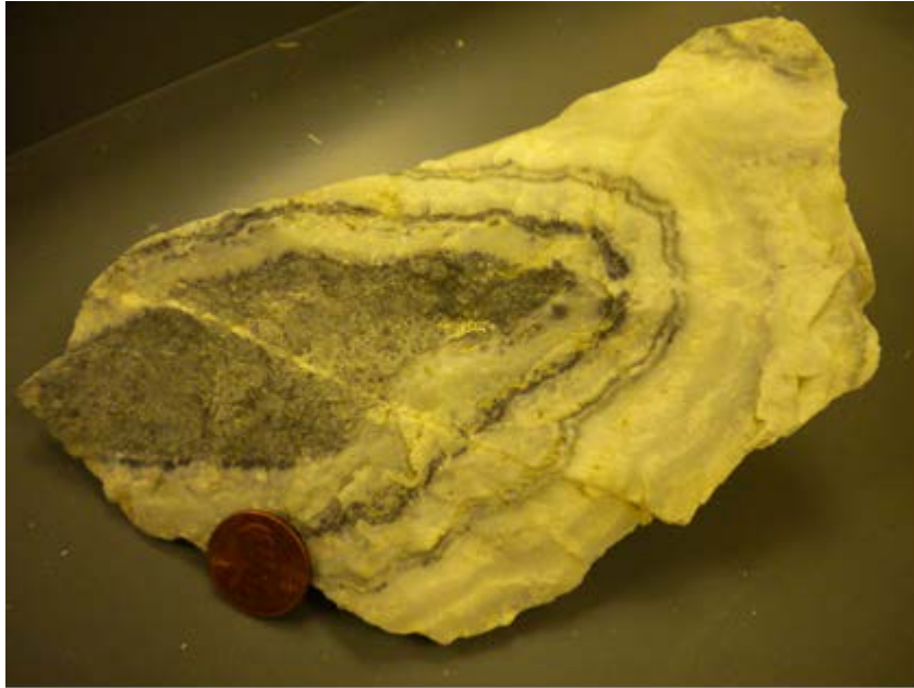
Figure 1. Hand specimen photograph of typical epithermal crustiform texture in the Midas district. Basalt is encrusted in the center of the sample (sample provided by Dr. James Saunders; photography by Rue Anne Chitwood, 2011).
