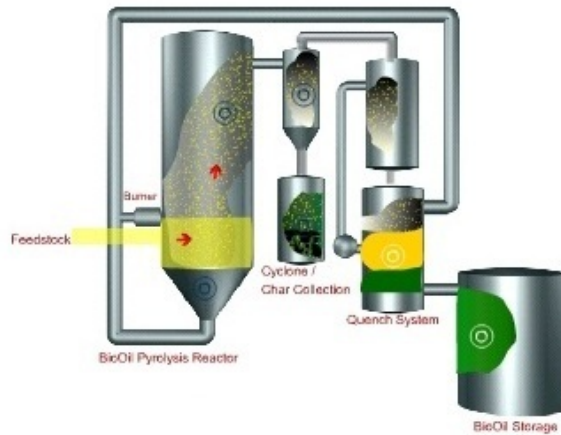
Figure 2.4: Schematic of a pyrolysis reactor (Jacquot, 2007)
