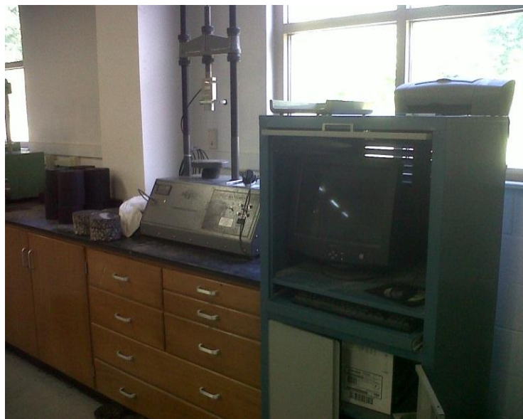
Figure 4.3: S5840 Geotest Loading Machine for Indirect Tensile Strength
