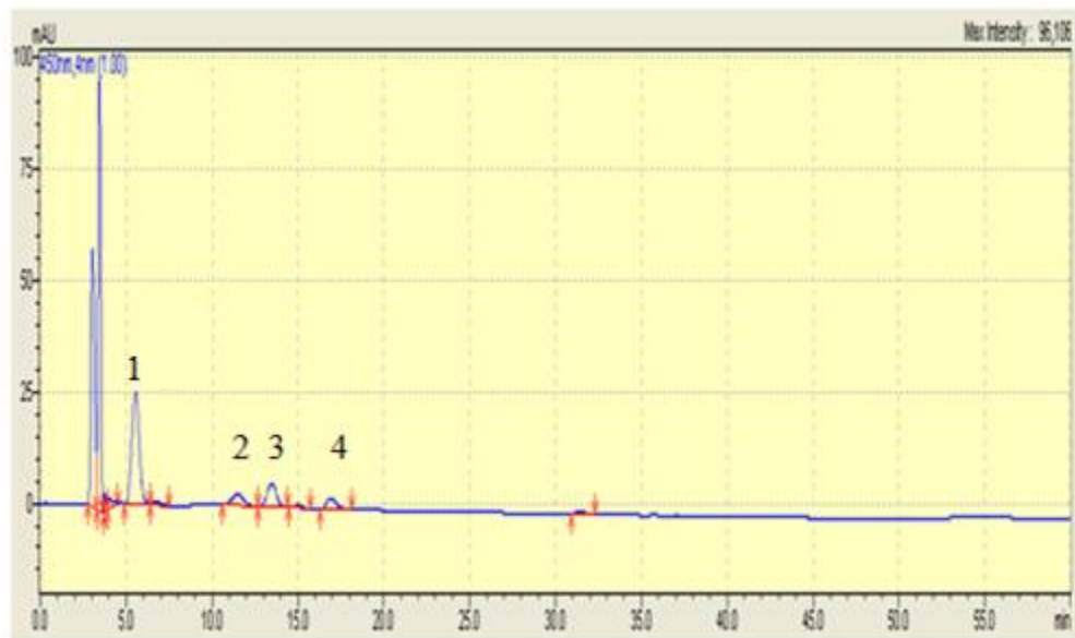
Fig D.1-HPLC chromatogram (absorbance at 450 nm vs. retention time) of carotenoids extracted from channel catfish fillets. Peak 1: Sudan I; Peak 2: Lutein; Peak 3; Zeaxanthin; Peak 4: Alloxanthin.
