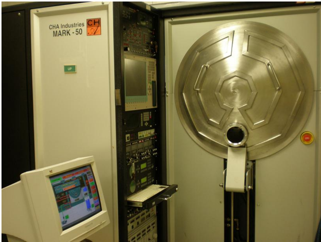
Figure 2.5. CHA Mark-50 deposition system: The CHA industries Mark 50 E-beam deposition system allows electrode deposition of 33 wafers measuring 100 mm (4") diameter in one run. Fifty nm of titanium was first deposited, followed by 200 nm of gold to form the electrodes.
