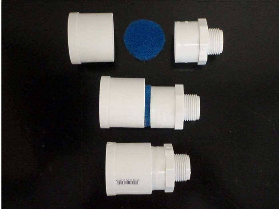
Fig. 1. Photo detailing drain components.
