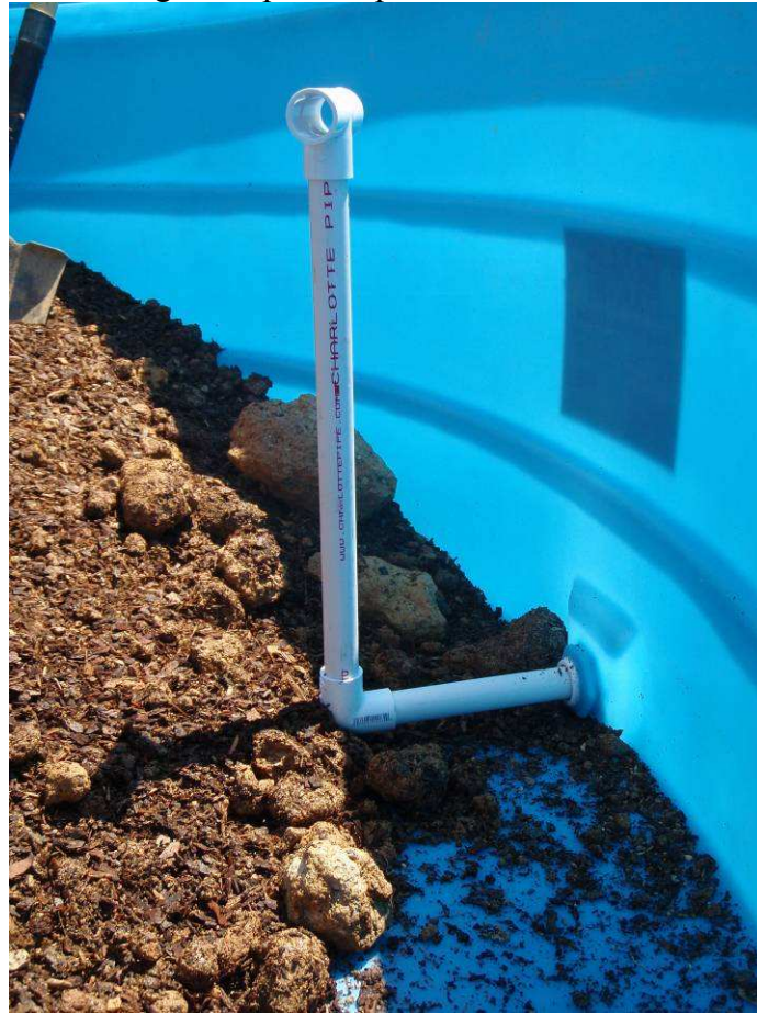
Fig. 2. Photo depicting tank fitted with overflow pipe for above-ground pond experiment.
