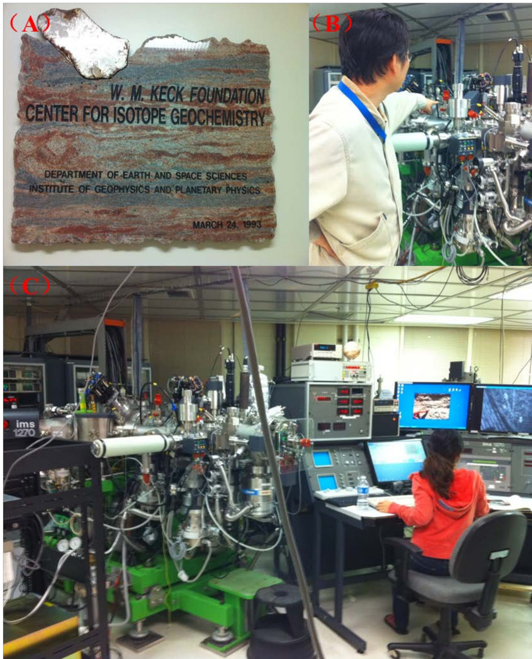
Figure 15. Photograph of the CAMECA ims 1270 at the NSF National Ion Microprobe Facility at the University of California, Los Angeles (UCLA). (A) Lab plaque; (B) Sample chamber area; (C) User operating area.
