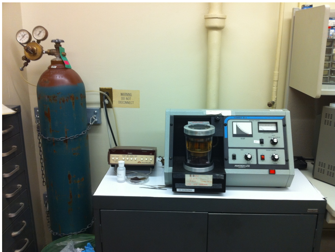
Figure 14. Photograph of Gold Coater at the NSF National Ion Microprobe Facility at the University of California, Los Angeles (UCLA). The Gold Coater is used to coat a mount with gold served as electrically conductive surface to make contact with the lip on the sample holder.
