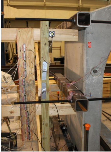
Figure 3-15: Detailed View of Laterally Restraining HSS Sections Installed
