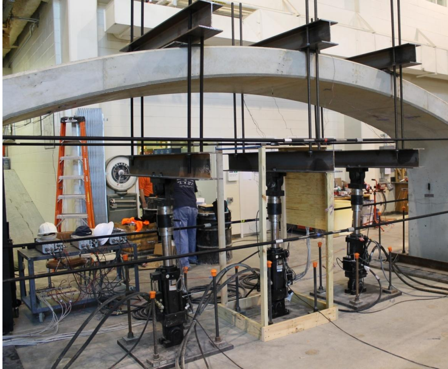
Figure 3-12: Loading Actuator Configuration
