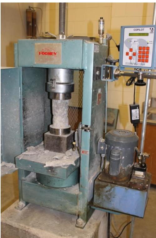
Figure 4-3: Concrete Cylinder Test
