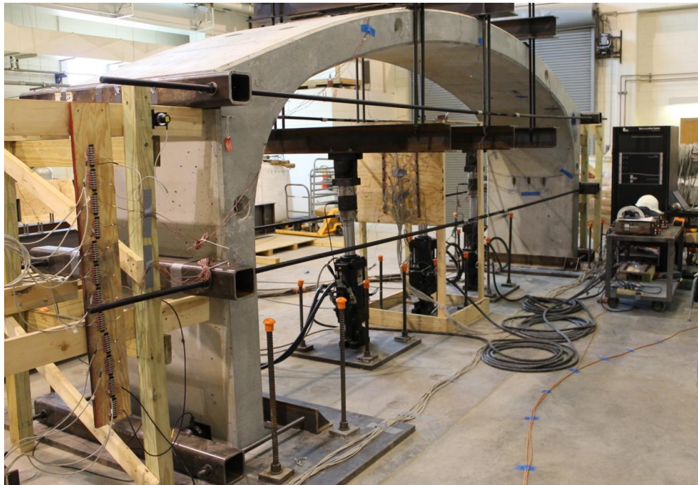
Figure 3-14: Structure with Lateral Restraint System Installed
