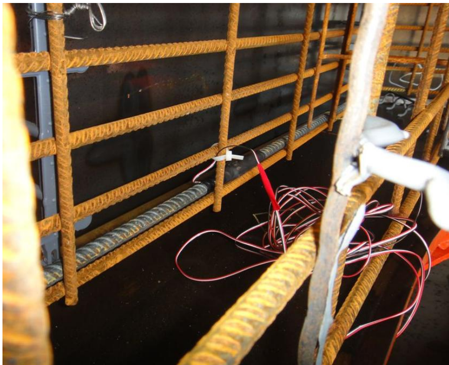
Figure 3-9: Securing Wires of Strain Gauged Reinforcing Bar
