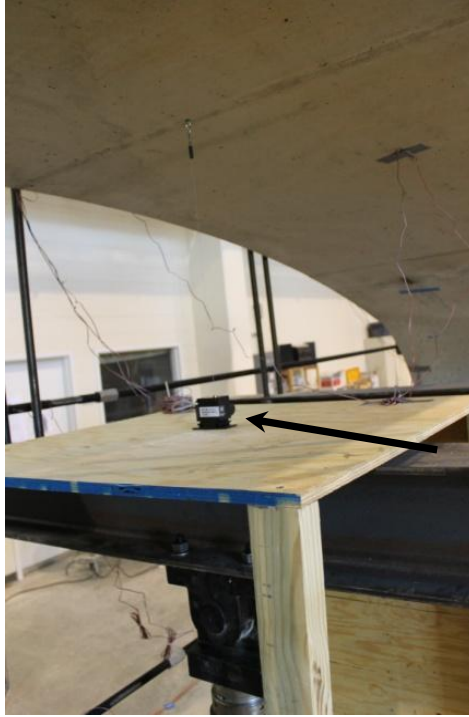
Figure 3-10: Midspan Wire Pot Deflection Gauge Installed
