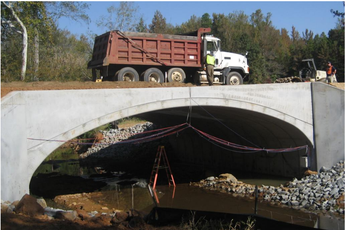
Figure 3-3: Field Testing – Three Axle Dump Truck at Midspan
