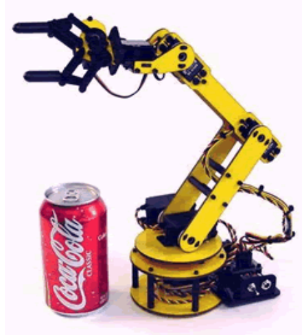
Figure 4.3: Lynxmotions Lynx6 Arm
