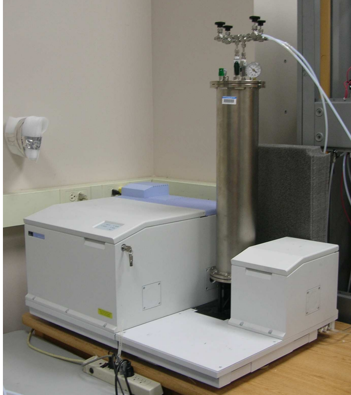
Figure 3.4: FTIR gas analysis chamber from the sensor evaluation system.
