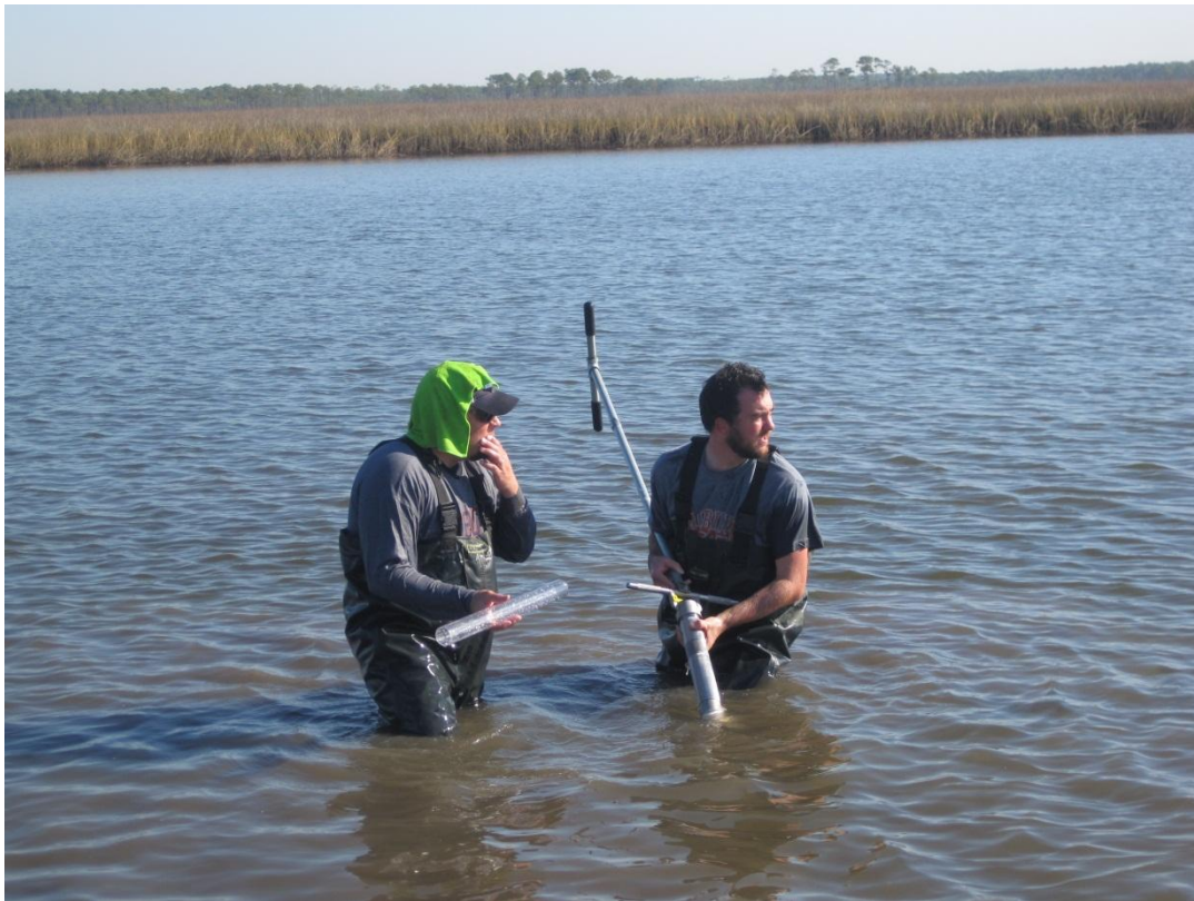
Figure 2. Photograph of sediment coring and surface-water sampling at Bayou Heron (BH), Mississippi.
