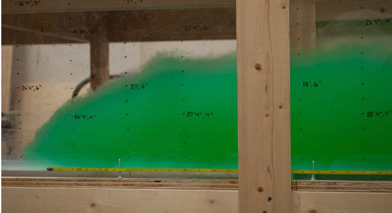
Figure 4.4: Photograph of the leading edge of a GC that illustrates the procedure in which the front trajectories were measured.
