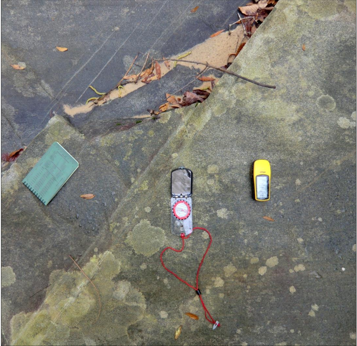
Figure 12. Example of the instruments used during fieldwork. From left to right: field notebook, geologic compass, GPS. Rock outcrop is on the southeastern rim area of Wetumpka impact structure.
