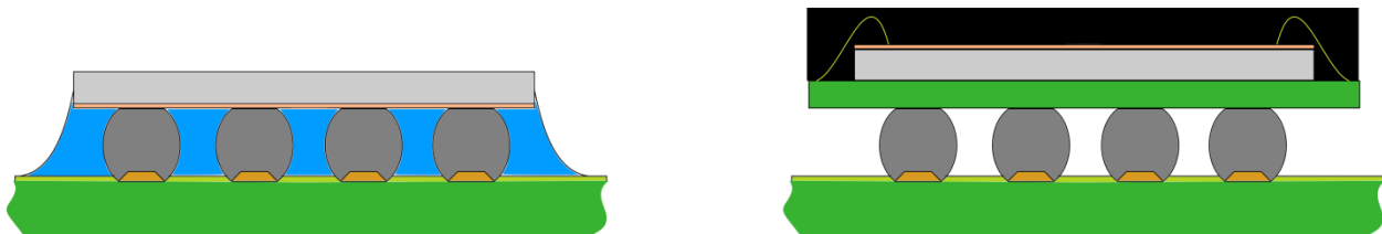
Figure 6: Cross section of a flip chip package (left) and a BGA package (right)
