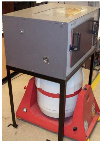
Figure 191: Thermal chamber with upper window mounted on top of the shaker table
