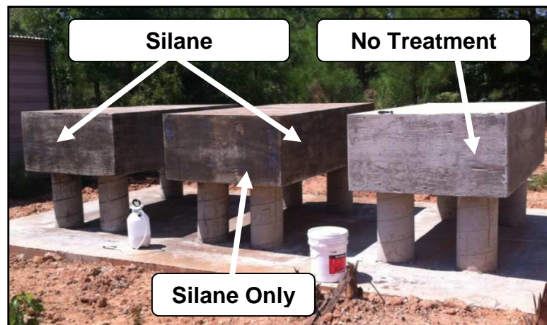
Figure 7.19: Silane application on arch test section
