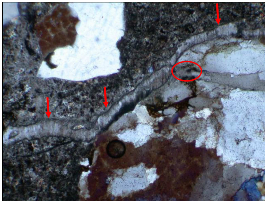
Figure 3.14: Core 1A – South: Microcracks filled with ettringite, shown with arrows. Small amount of gel at outside edge of crack in aggregate is circled.
