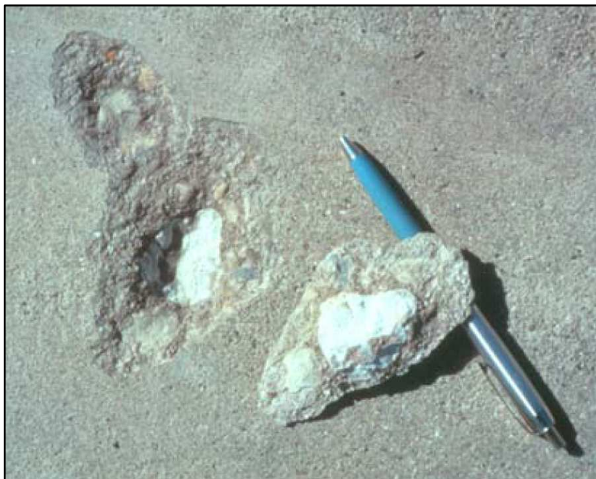
Figure 2.12: Example of a pop-out induced by ASR (Fournier et al. 2004)
