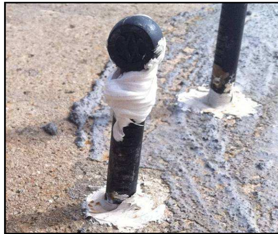
Figure 5.1: RH tube with plug installed and tube sealed with a flexible silicone sealant
