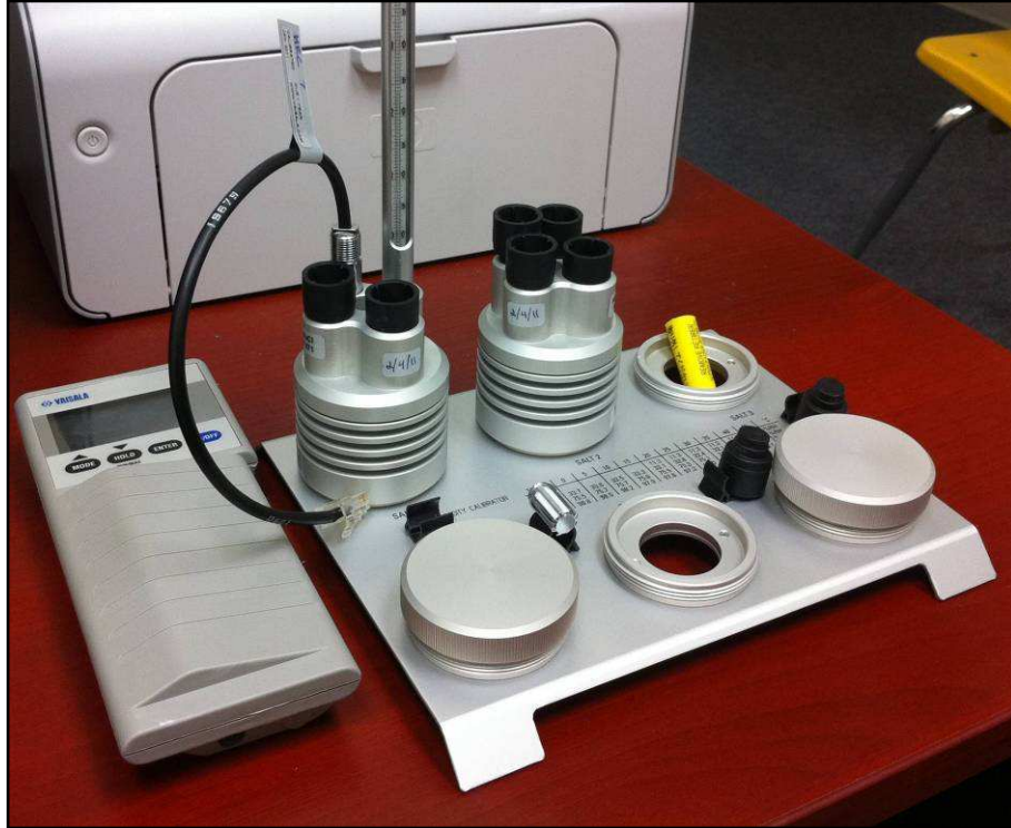
Figure 5.7: Vaisala's Humidity Probe Calibrator, HMK15
