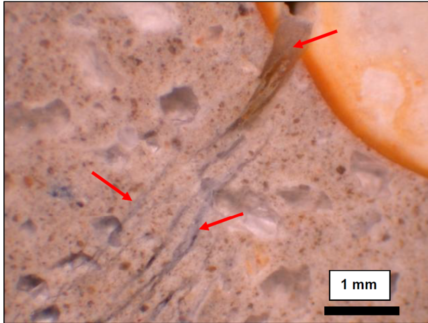
Figure 3.13: Crack at periphery of quartzite aggregate particle (top right) and multiple veinlets, indicated with arrows, filled with ASR gel (WJE 2010)
