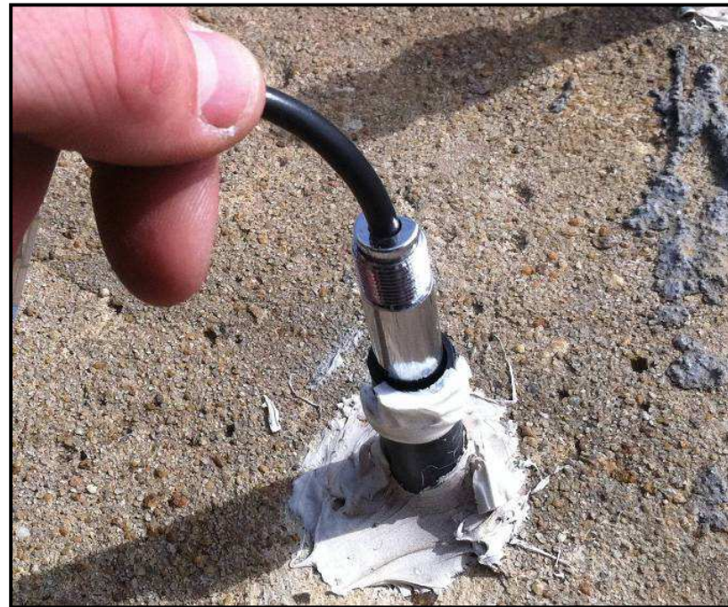
Figure 5.3: RH probe being inserted into tube
