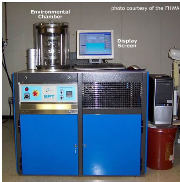
Figure 3-5 Asphalt Mixture Performance Tester (85).
