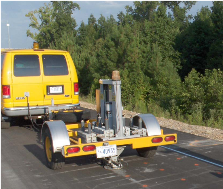
Figure 3-11 Falling Weight Deflectometer.
