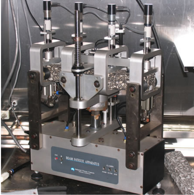
Figure 3-9 Beam Fatigue Apparatus (85).
