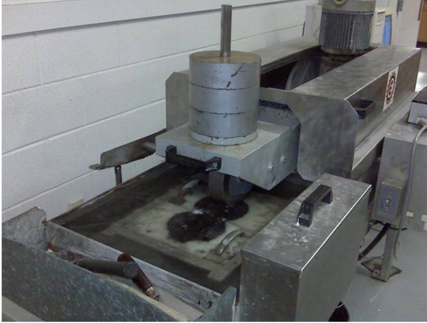
Figure 3-7 Hamburg Wheel Tracking Device.
