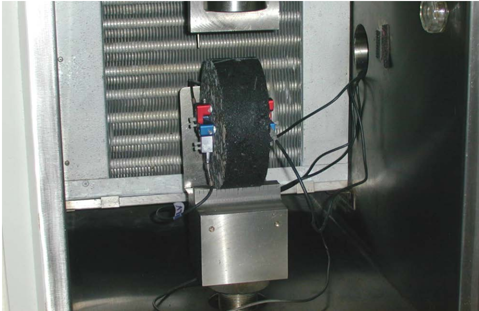
Figure 3-10 Indirect Tension Test Setup (92).
