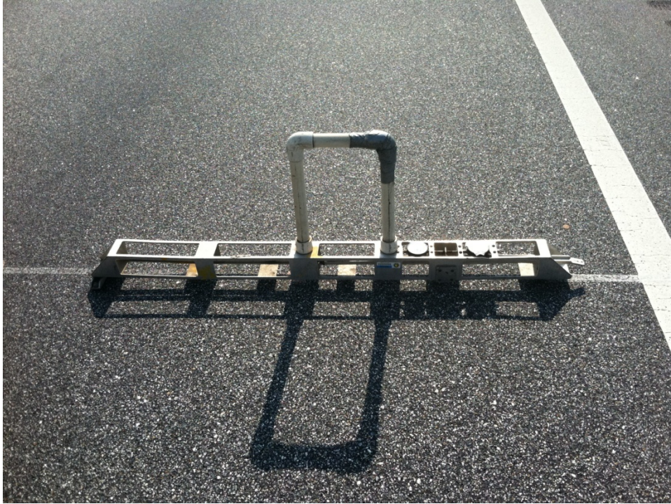
Figure 3-13 ALDOT Rut Depth Gauge Method.
