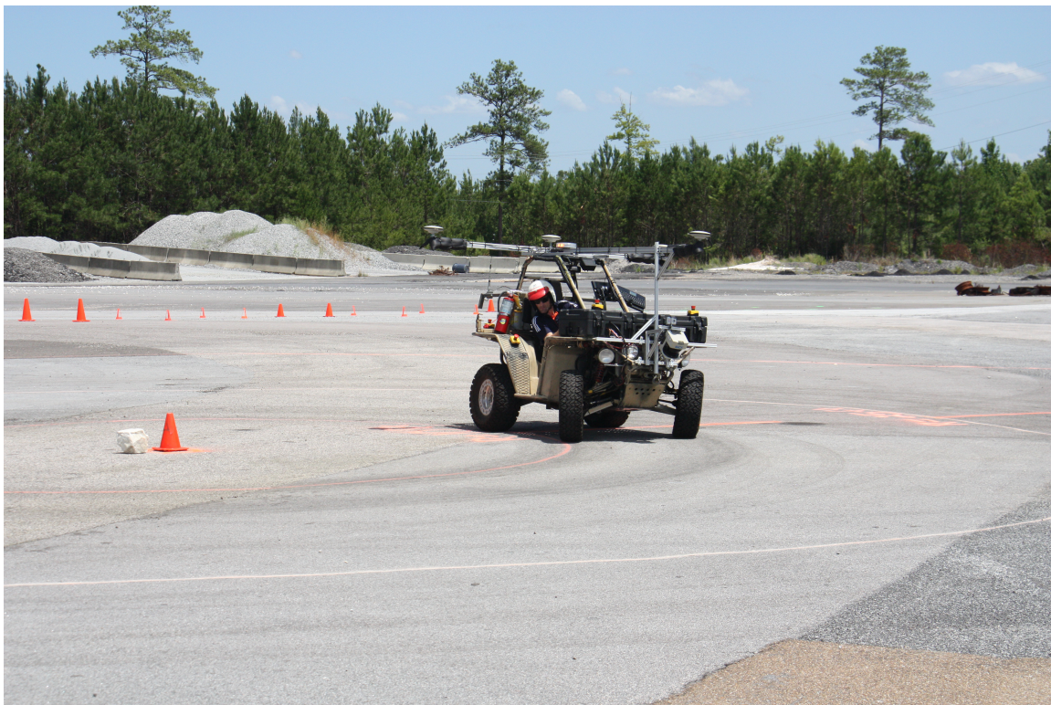
Figure 7.25: Tire Relaxation and Asymmetrical Steering
