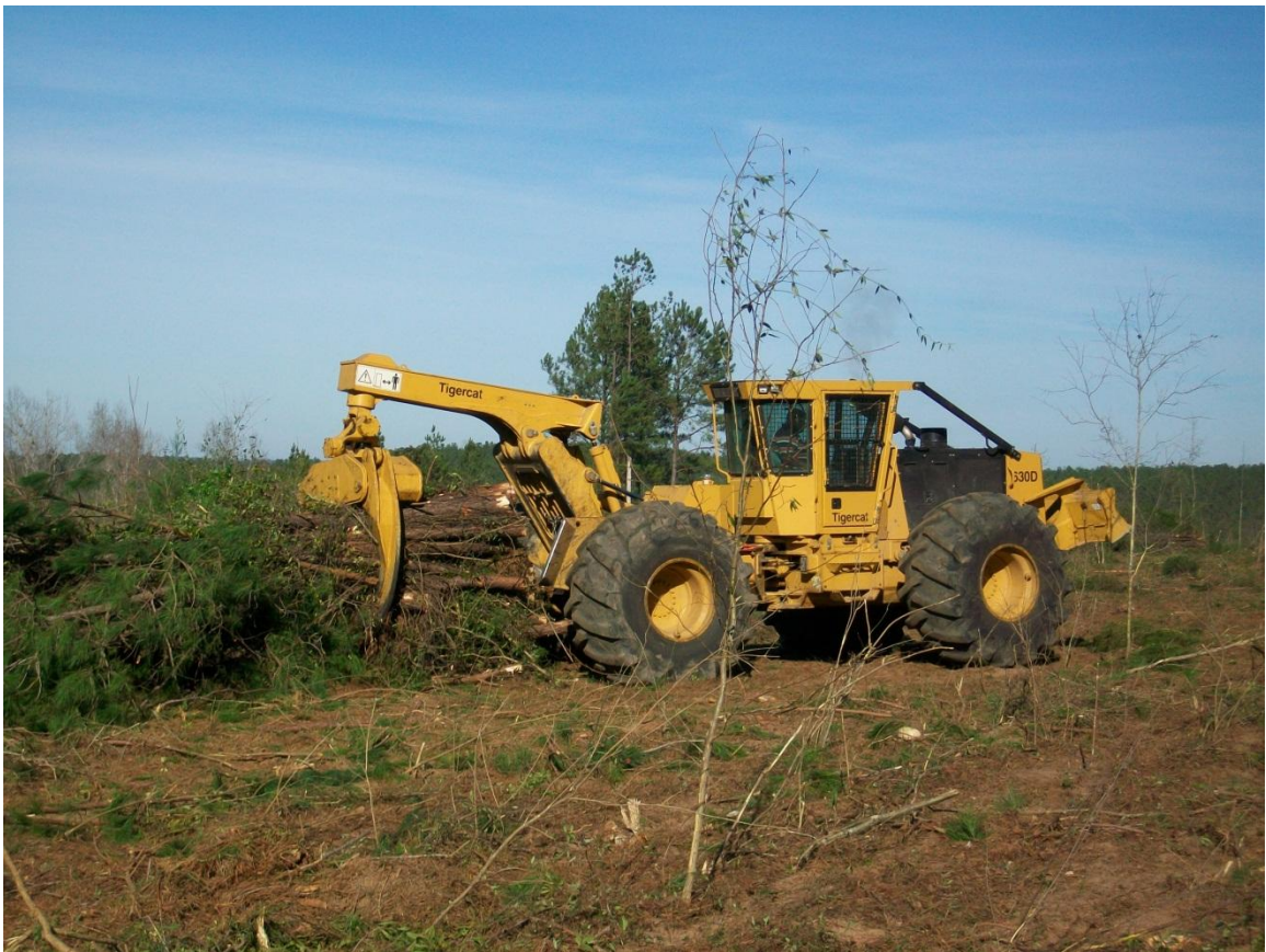
Figure 11: Tigercat 630D traveling towards the landing with a full payload.
