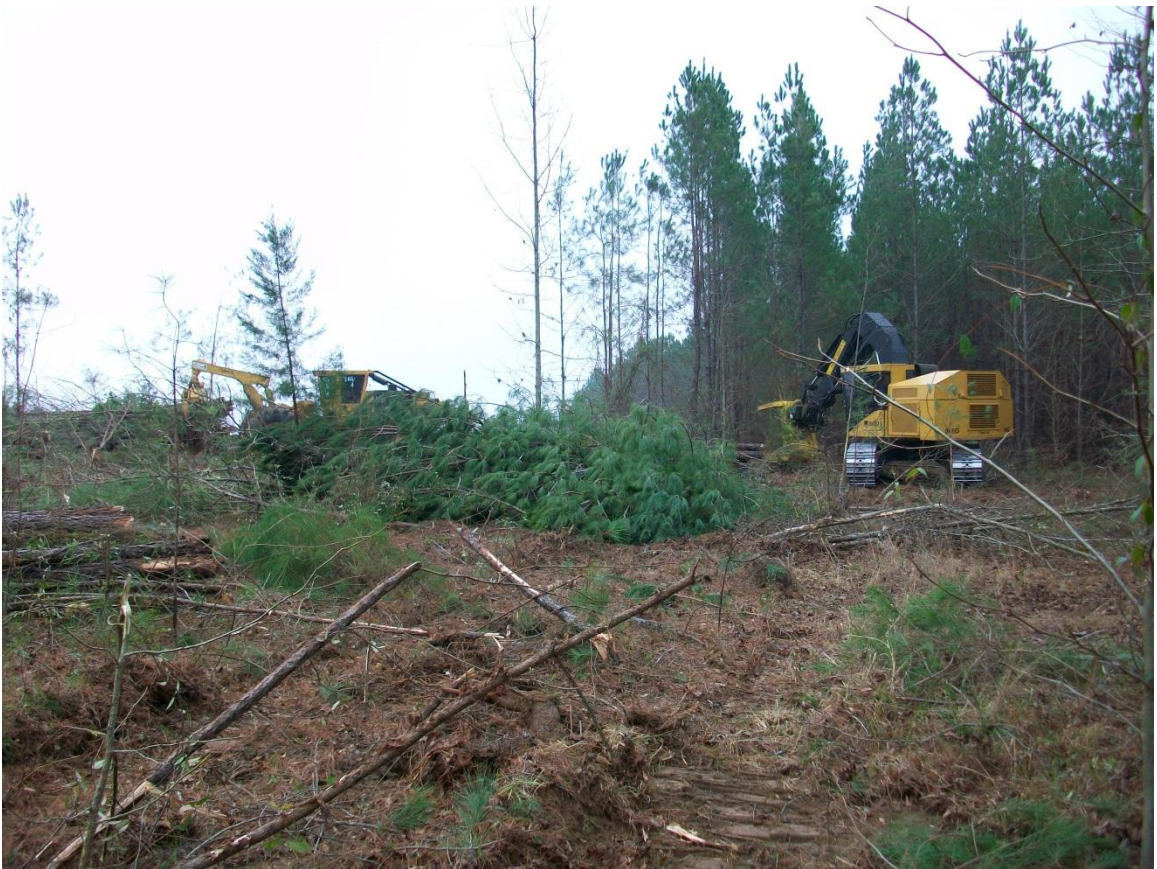
Figure 15: Feller-buncher and skidder working near one another during the study.
