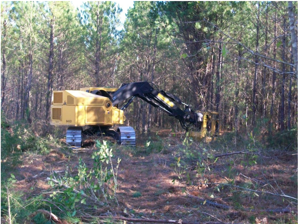
Figure 9: Tigercat 845D with a full accumulation of pine stems.
