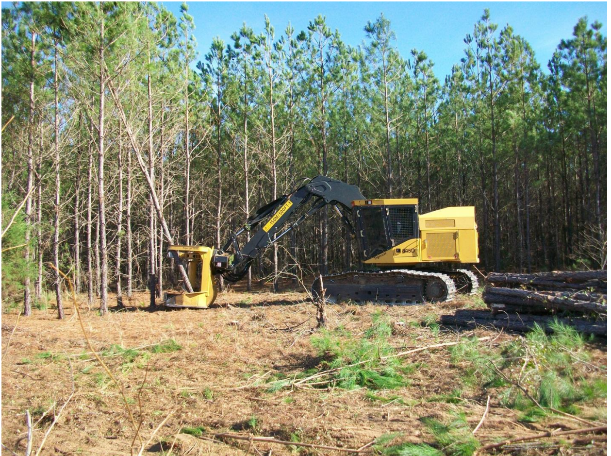
Figure 2: Tigercat 845D equipped with specialized biomass shear head.
