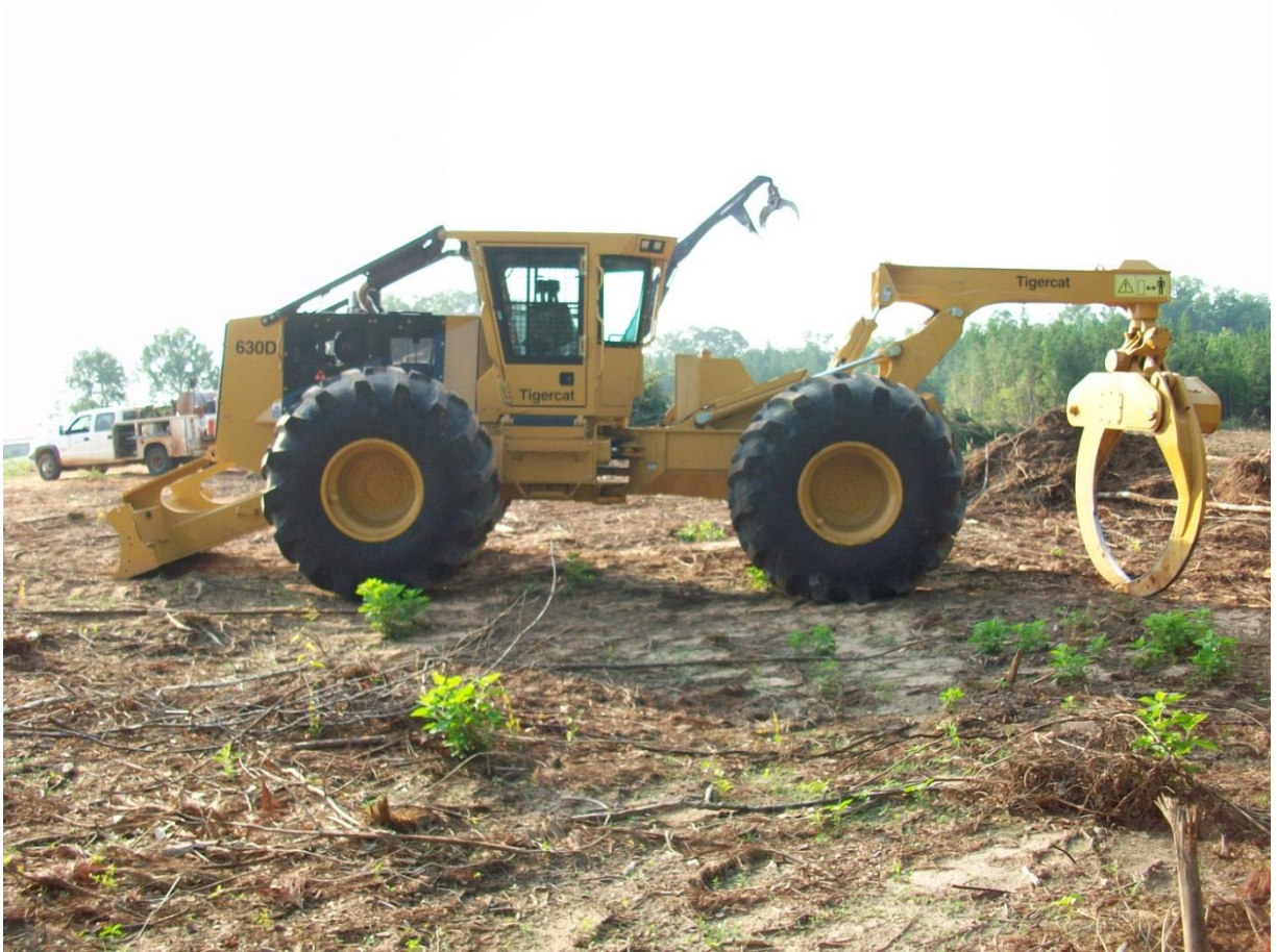
Figure 5: Tigercat 630D skidder with oversized grapple.
