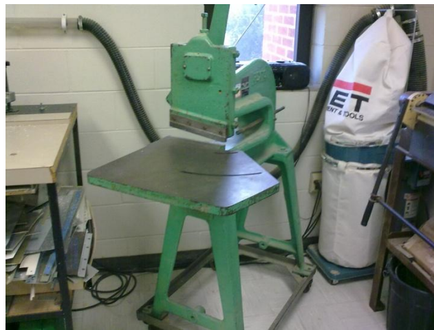
Figure 83. Hand Shear Used in Preparing Off-Axis Test Specimens
