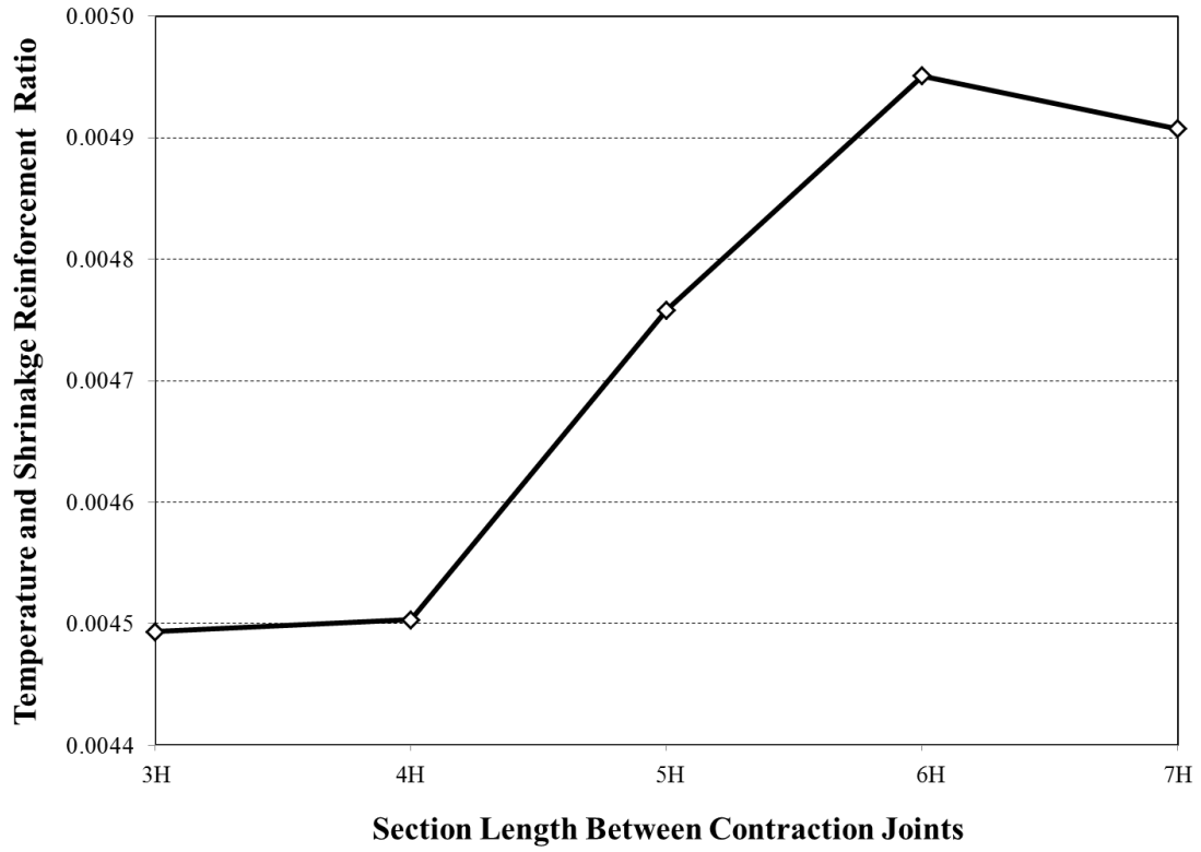
Figure 4-6: Temperature and Shrinkage Reinforcement Ratio versus Section Length between Joints to Keep the Average Crack Width of AEB Culvert at 240+37 at 0.012 in. (0.30 mm)
