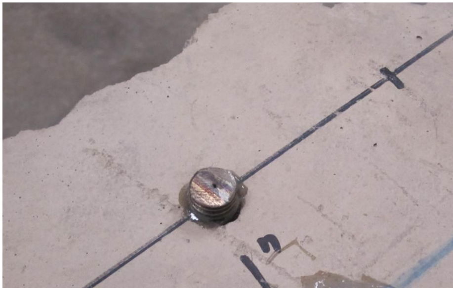
Figure 5-5: DEMEC Stud Installed in Concrete
