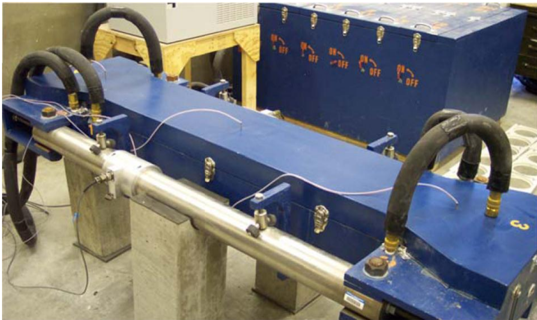
Figure 5-12: Rigid Cracking Frame at Auburn University
