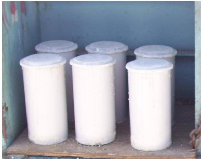
Figure 3-11: Tarp-Cured Test Specimens in Molds with Plastic Caps
