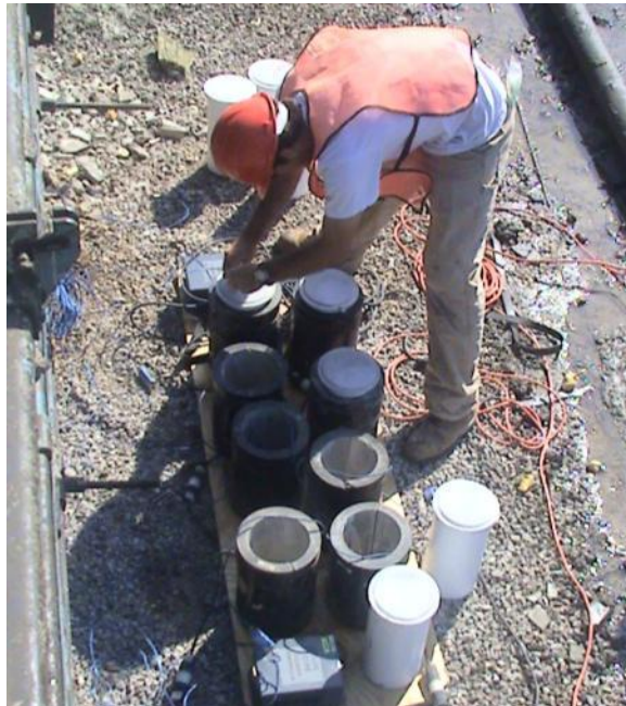
Figure 3-14: Inserting Test Cylinders into Match Curing System
