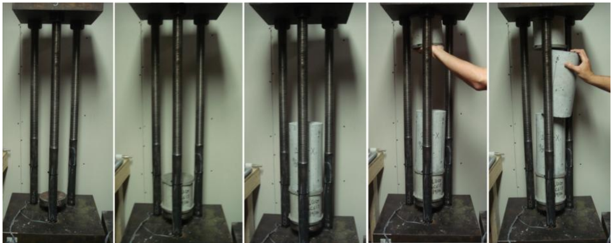
Figure 3-31: Example of Loading the Creep Frames
