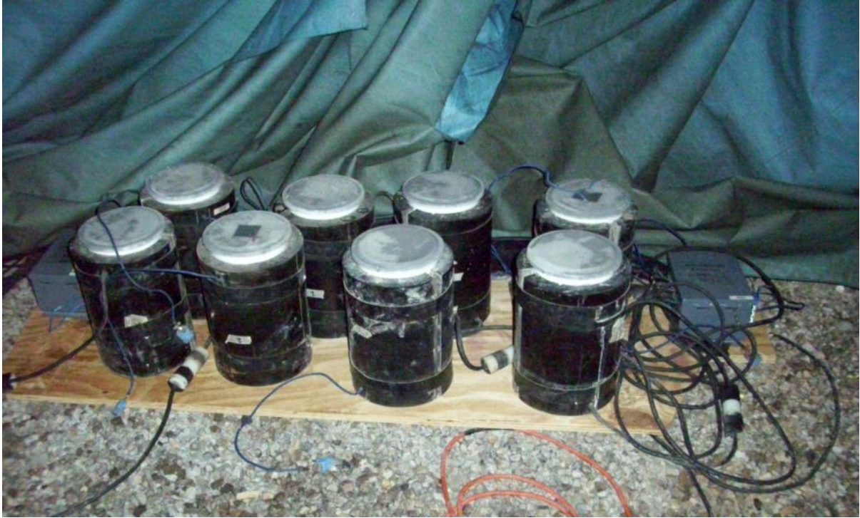
Figure 3-18: Match Curing System Alongside Tarp-Covered Girder
