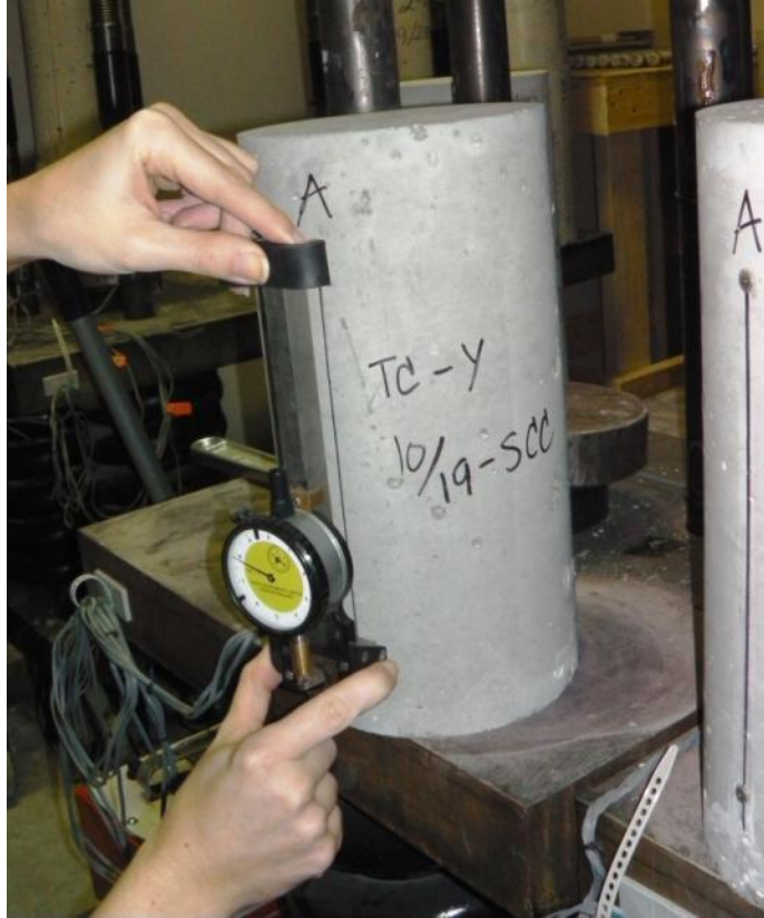
Figure 3-40: Taking Shrinkage Strain Measurements Using DEMEC Gauge
