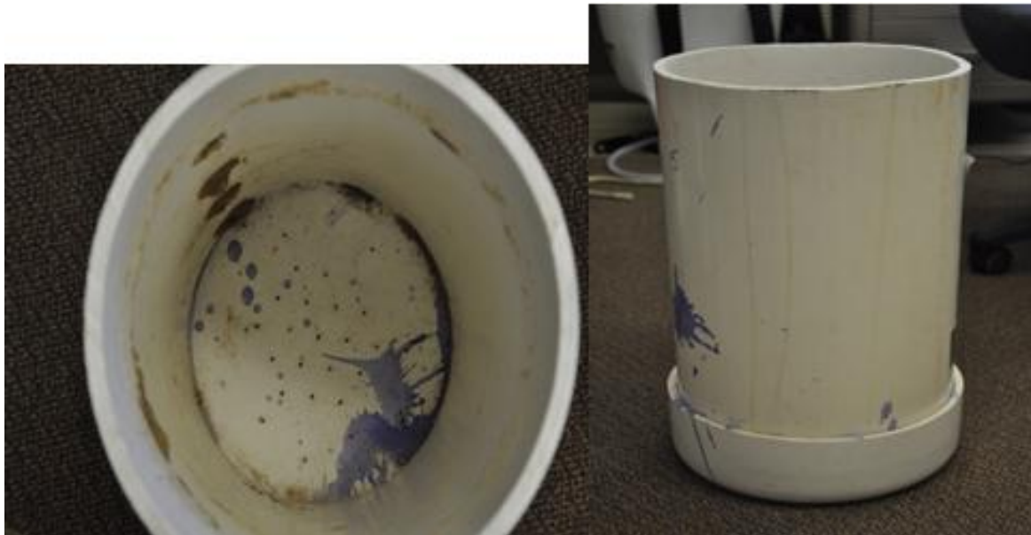
Figure 2.2 PVC test arena showing height (45.2 cm), bottom cap, and drainage holes
