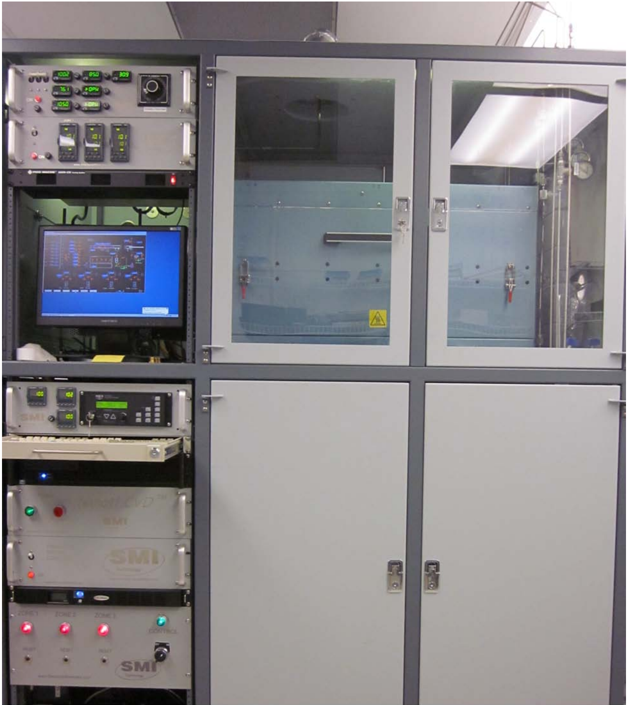
Figure 3.3(a): LPCVD system (NanoH CVD TM ) used to deposit SiO 2 on SiC.
