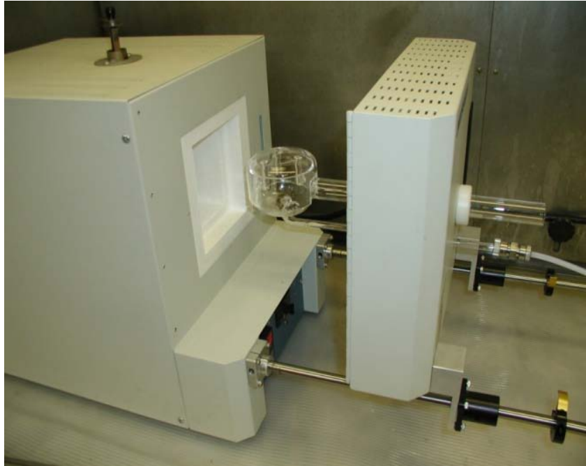
Figure 4.1(a): A planar diffusion source (PDS) furnace.
