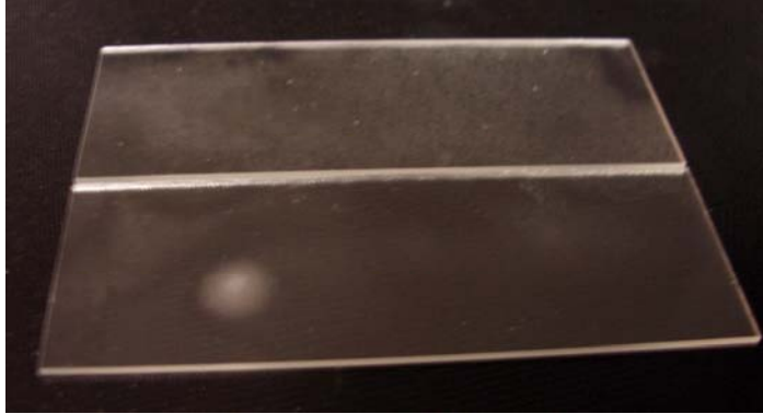
Figure 2.9 – Polyethylene film alone (top) and polyethylene film with underlying RDX film (bottom) placed on a glass slide.
