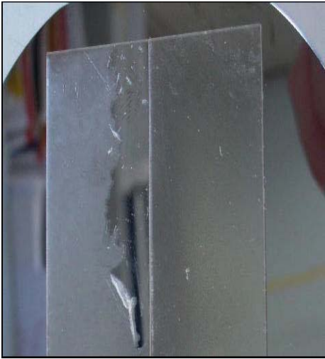
Figure 2.7 - Polyethylene films sprayed at room temperature (left) and at \sim 100\text{ }^{\circ}\text{C} (right).
