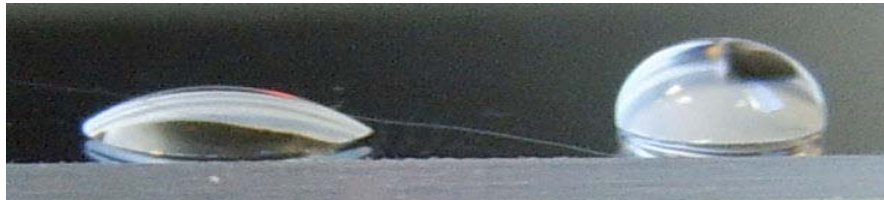
Figure 2.1 – Water droplets placed on a microscope slide covered with polycarbonate film (right) and on a droplet placed on a microscope glass slide without film (left).
