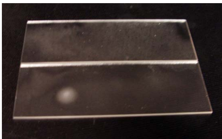
Figure 2.11 - Polycarbonate film alone (top) and polycarbonate film with underlying RDX film (bottom) placed on a glass slide.
