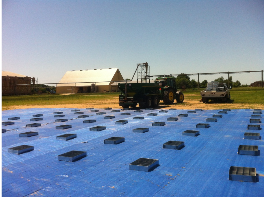
Figure 20. Pan array for BB particle trajectory tests.
