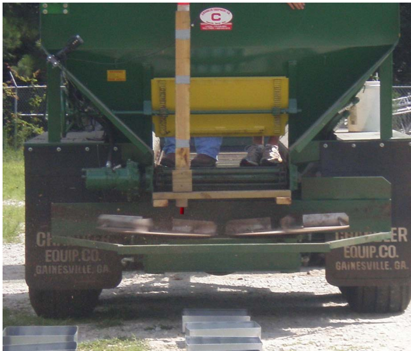
Figure 17. PVC pipe and funnel assembly attached to litter spreader for BB particle trajectory testing.
