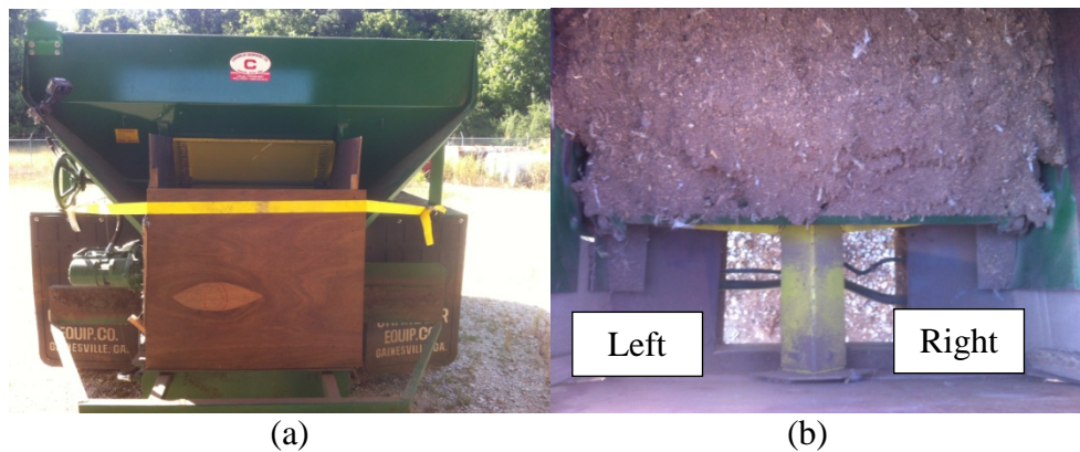
Figure 22. Wooden box (a) used to funnel litter that fell on each side of the flow divider (b) into two collection bins.
