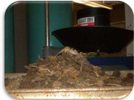
Large X > 4.75 mm ASTM No. 4 sieve
