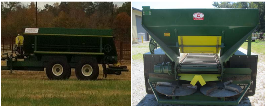
Figure 10. Chandler Equipment Co. litter and shavings spinner-disc spreader.
