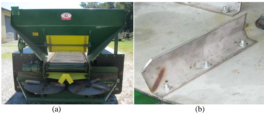
Figure A.2. (a) Litter spreader rear gate, conveyor chain, flow divider and spinners; (b) Vane used on each spinner-disc.
