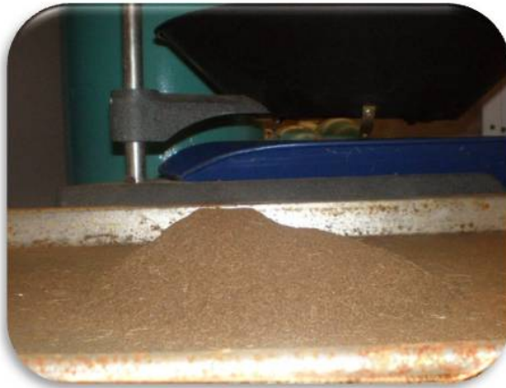
Small X < 0.42 mm ASTM pan
