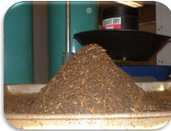
Medium 0.42 \text{ mm} < x < 4.75 mm ASTM No. 40 sieve
