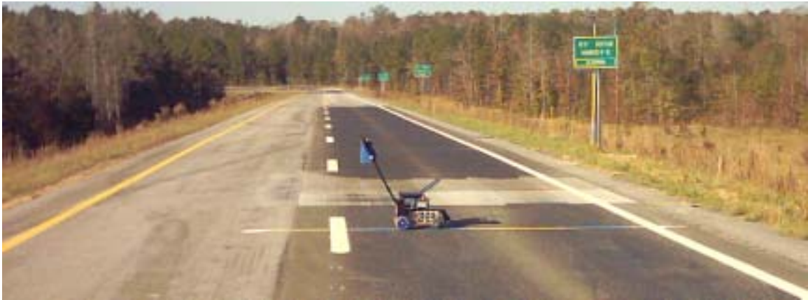
FIGURE 4.3 Dipstick Elevation Measurements Along Transverse Test Location.
