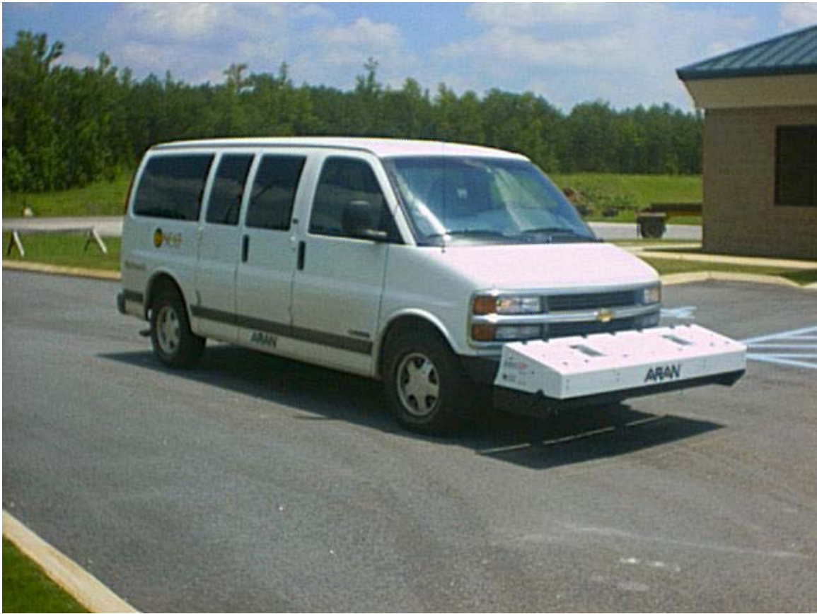
FIGURE 4.1 Auburn University's High Speed Inertial Profiler Used to Make Continuous 3-Point Rut Measurements.
