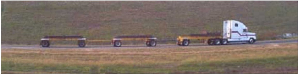
FIGURE 3.9 Triple Trailer Rig Used to Apply Accelerated Loading.
