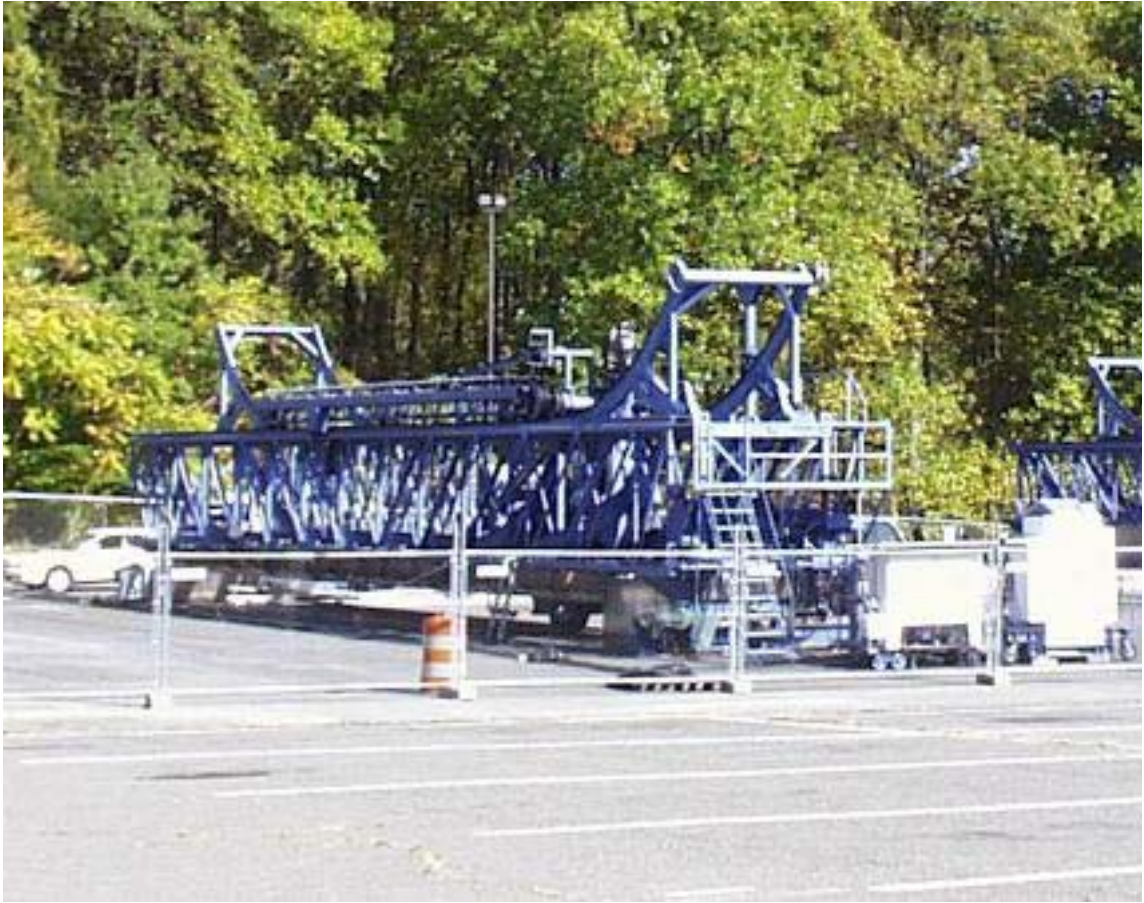
FIGURE 2.4 Later Load Simulator Testing via ALF at FHWA's PTF.
