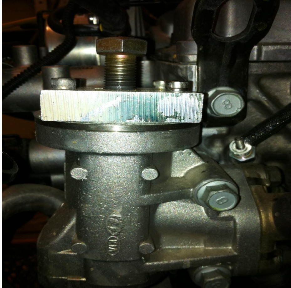
Figure 4-4: EGR Control Apparatus
